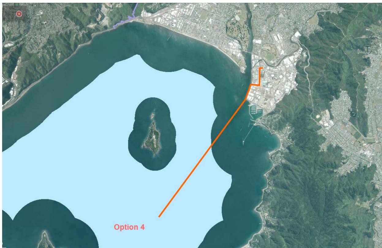
Figure 1-2: Seaview wastewater outfall option 4
