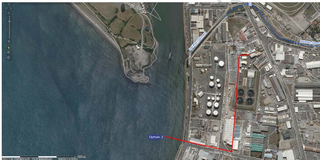
Figure 4-3: Location of Seaview wastewater outfall option 3
