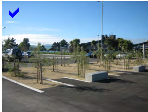
Shading structures, trees, shrubs and appropriate paving minimise the visual impact of surface car parking. Areas of porous paving and vegetation are encouraged to reduce urban water runoff
