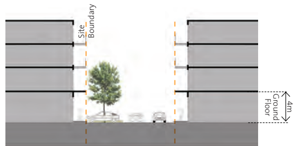
Option for street layout: Buildings are set back 2.5m to allow for a footpath and angle parking.
