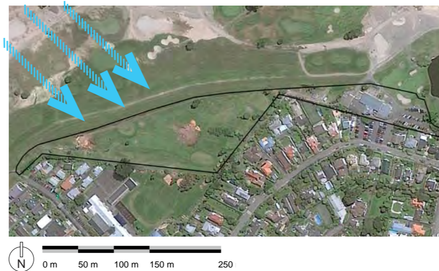
Fig 3.1.12 The site is exposed to the prevailing nor-westerly winds. The site opens towards the north west, making the main body of the site particularly vulnerable to these winds.
