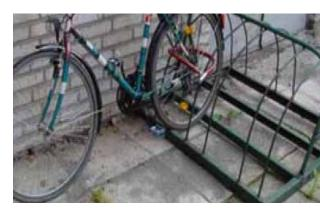
Wheel stands are common, but they do not support the bike, make it difficult to secure the bike frame, and can damage the wheel.
