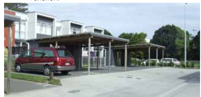
Communal parking at the rear allows buildings to front the street and minimises manoeuvring space for multi unit developments.
