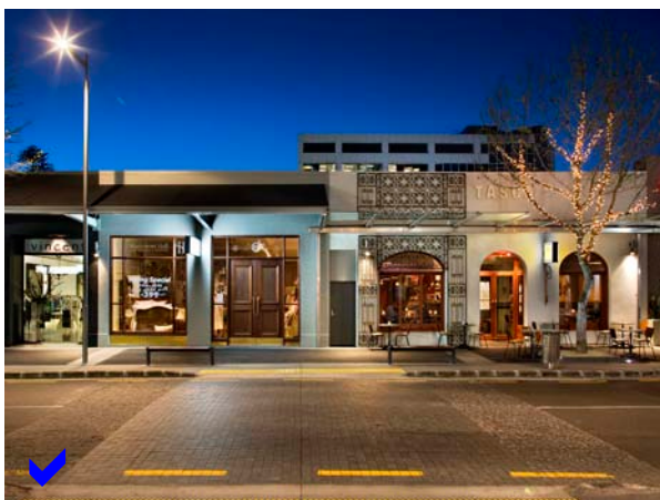
Long frontage modulated at intervals of less than 10m by change in uses (various shops and restaurants) materials, colours, good use of sheltering elements, high percentage of transparent glazing and public/private lighting
