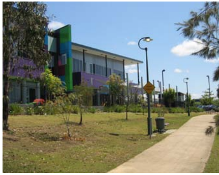
Pedestrian link and landscaped buffer separating uses through-visibility, public lighting, low and transparent fencing, windows overlooking the footpath. Projecting elements and different colours and materials reduce the bulky appearance of a large building.
