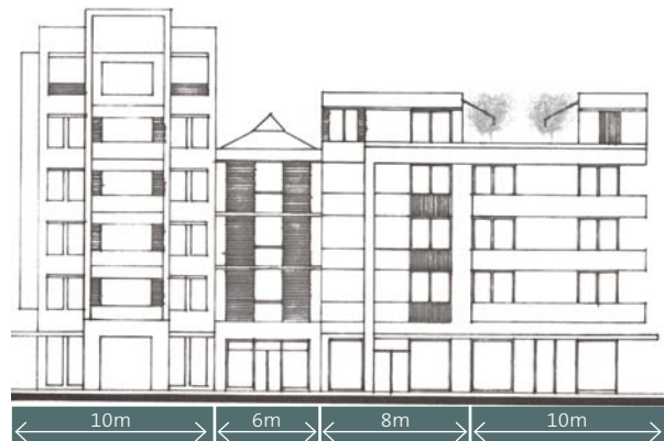
Example of a facade treatment in the Core Precinct. Long frontage lengths at intervals of less than 10m. Facade treatment of buildings (architectural elements and materials) on ground and upper floors at intervals of 2m to 6m to create interest to the streetscape.
