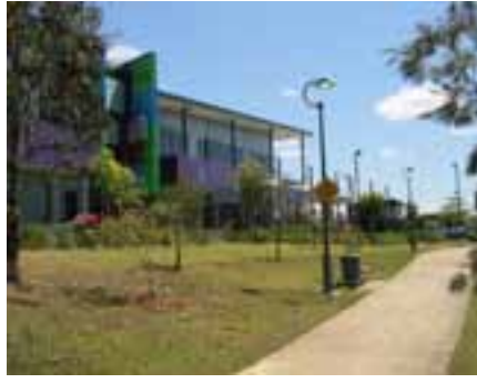
Pedestrian link and landscaped buffer separating uses, through-visibility, public lighting, low and transparent fencing, windows overlooking the footpath. Projecting elements and different colours and materials reduce the bulky appearance of a large building.
