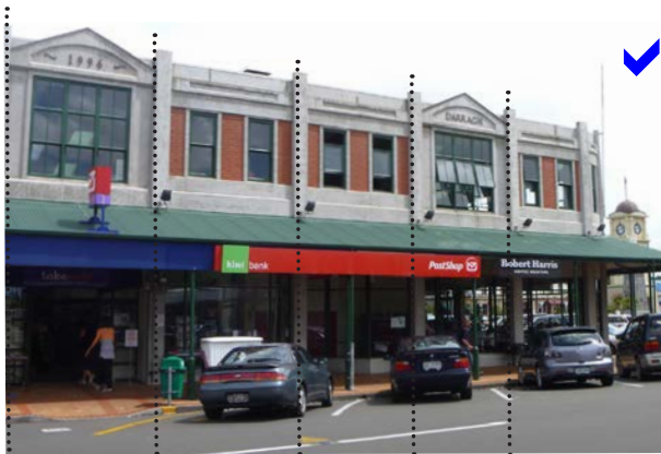
This building is a new block, but has an articulated form of identifiable parts given recessive and projecting elements (dotted lines). It is typical of the character of older buildings and a useful reference for new buildings.
