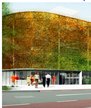
Green walls are a good solution to minimise the negative visual effects of car parking above ground within a large scale structure.
