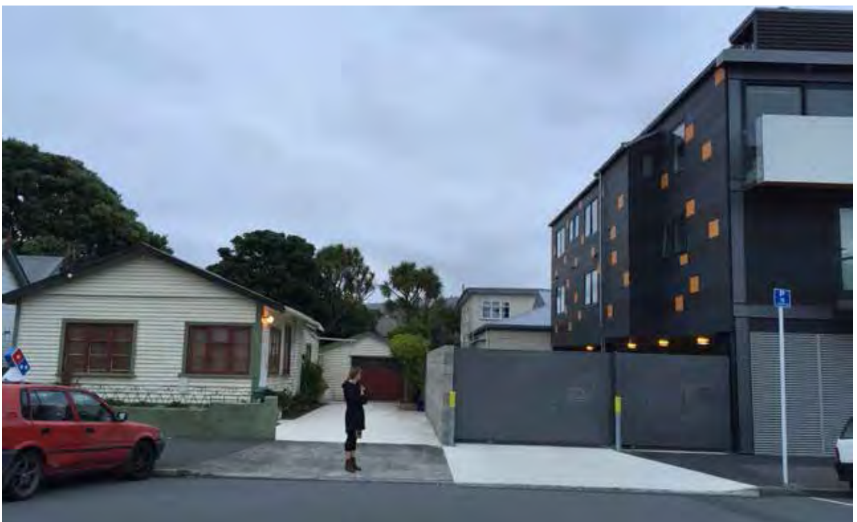
THE PHOTO ABOVE SHOWS THE TRANSITION FROM A LOW DENSITY, SINGLE STOREY BUNGALOW TO A MEDIUM DENSITY, THREE STOREY APARTMENT DEVELOPMENT AND THE BOUNDARY ISSUES THAT MAY RESULT. IN THIS EXAMPLE, ADDITIONAL MORNING SHADING IS EXPERIENCED BUT THE SETBACK REDUCES PRIVACY ISSUES
