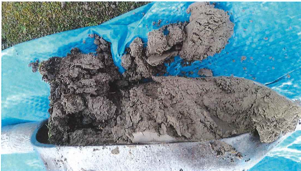
Photograph 6: Silty topsoil observed at a depth of 0.0 m bgl in HA16.
