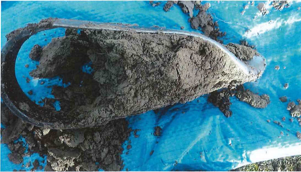
Photograph 7: Sandy silt observed at a depth of 0.25 m bgl in HA16.
