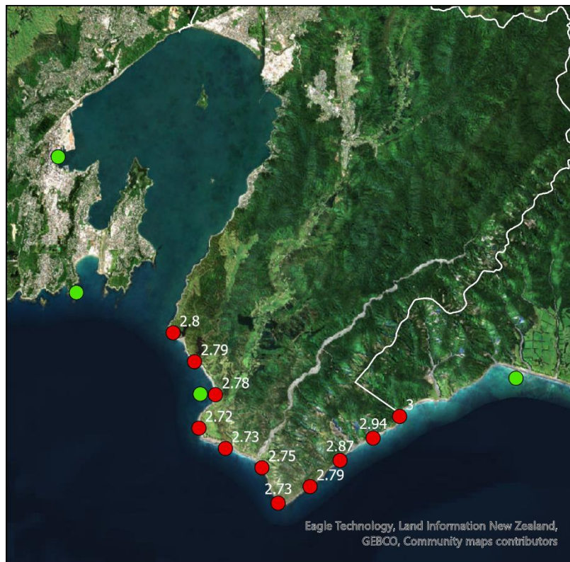
Figure 3-1: National inundation assessment locations and present-day 1%AEP inundation level (m NZVD). National assessment locations shown in green.
