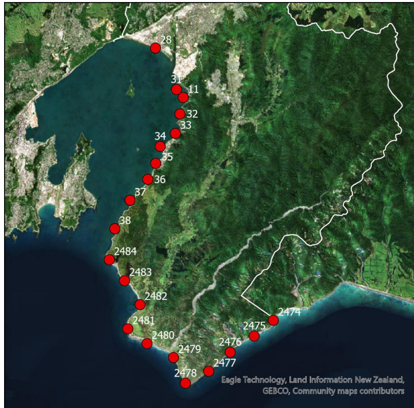
Figure 1-1: Reference locations used for extreme sea level and relative sea level rise analysis. White line is the Hutt City territorial boundary.
