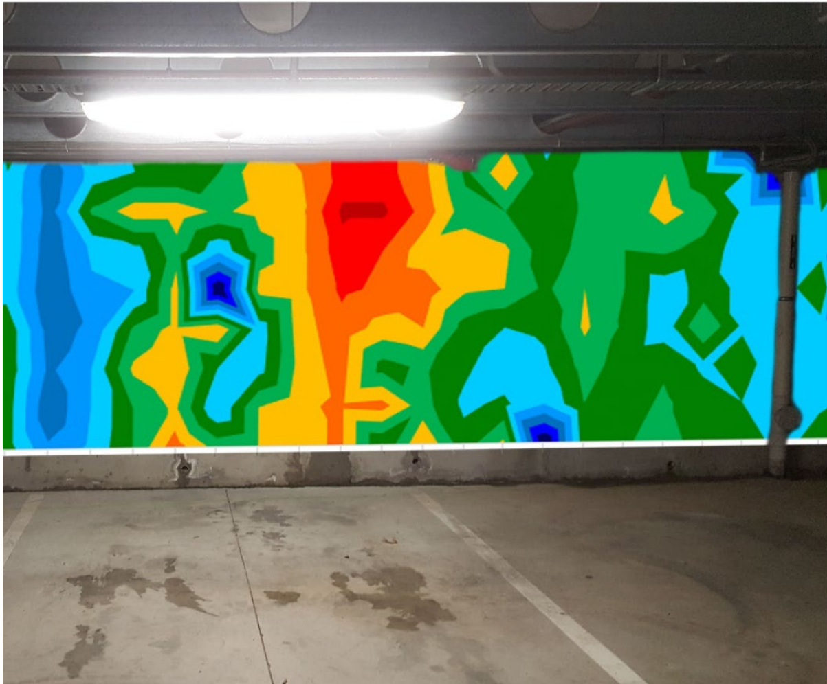
Figure 86: Example of half-cell Potential mapping
