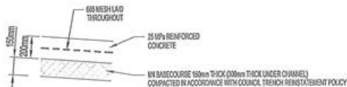
TYPICAL SLAB CROSS SECTION
