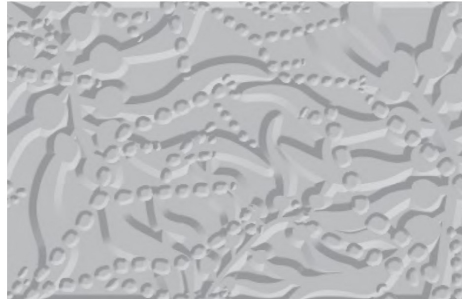
Figure 1.16 Indicative graphic of texture applied to curved seawalls horizontal surfaces and vertical faces
