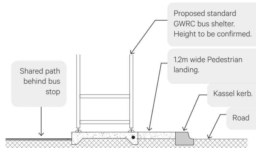
Figure 1.41 Typical bus stop side elevation showing level changes
