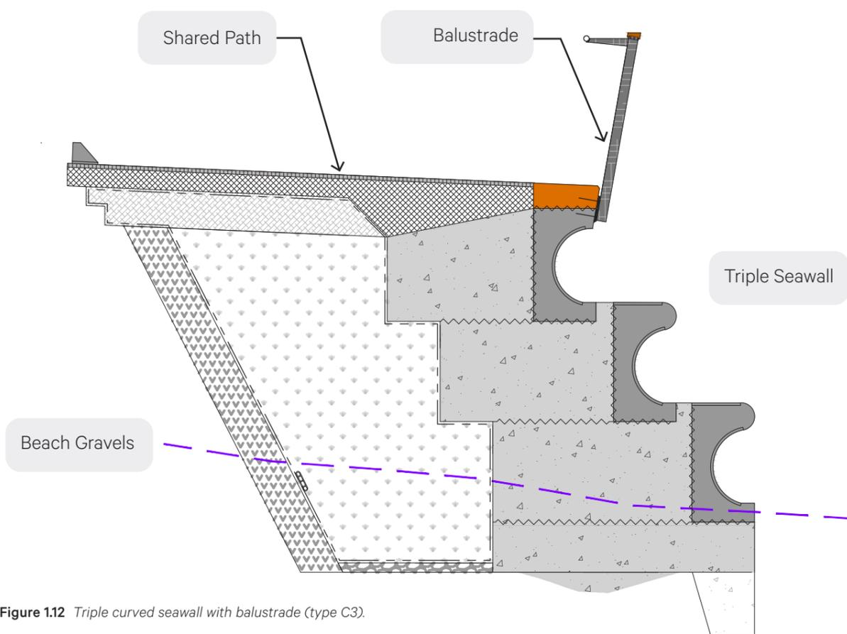
Figure 1.12 Triple curved seawall with balustrade (type C3).
