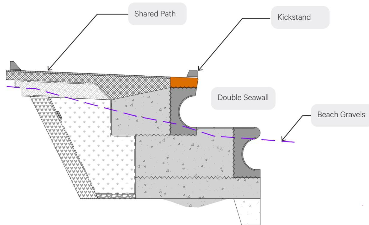
Figure 1.10 Double curved seawall with bench (type C2L).
