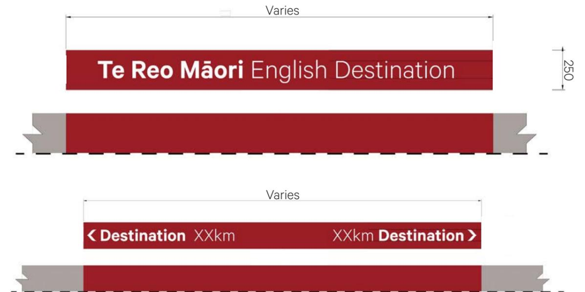
Figure 1.34 Steel panel with named location applied to kickrail (example only).
