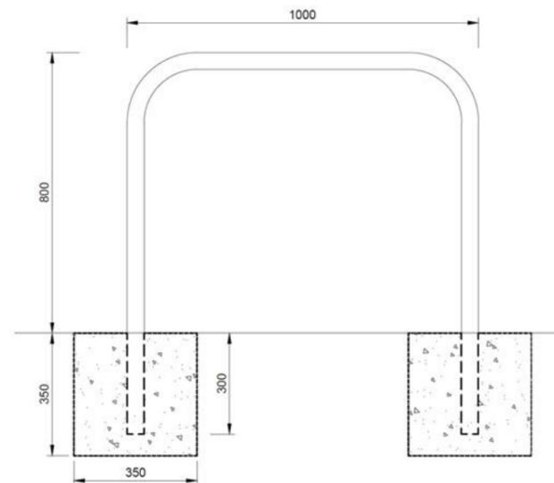
Figure 1.30 Typical cast in bike rack.
