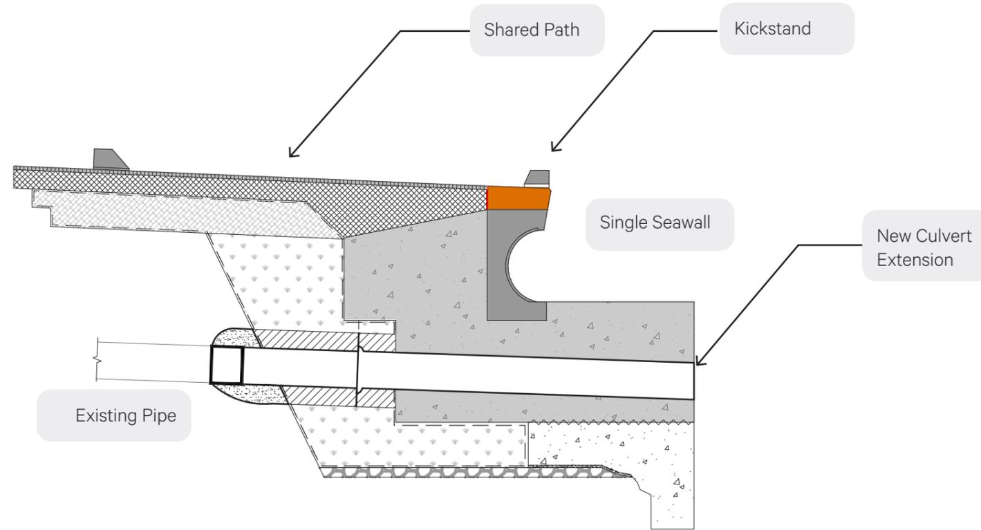
Figure 1.13 Single curved seawall with bench (type C1L) and stormwater outfall penetration.
