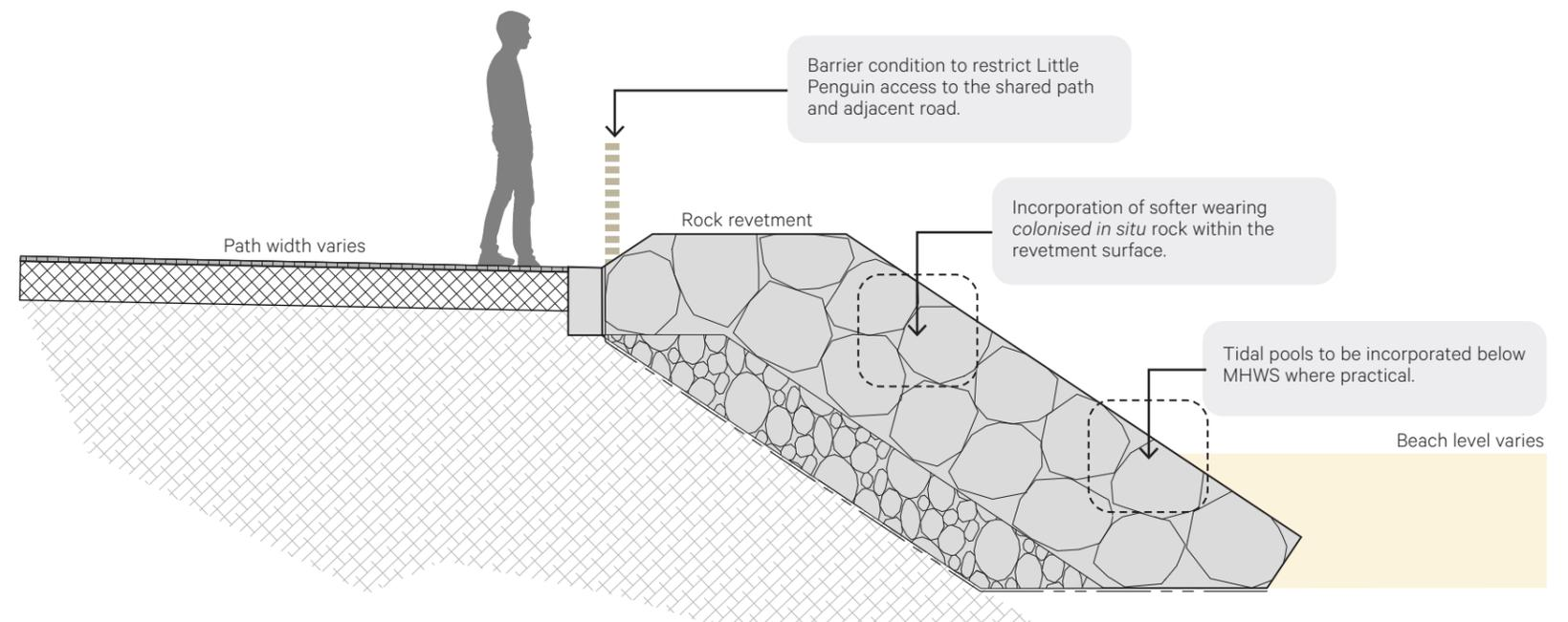
Figure 1.11 Typical rock revetment section.
