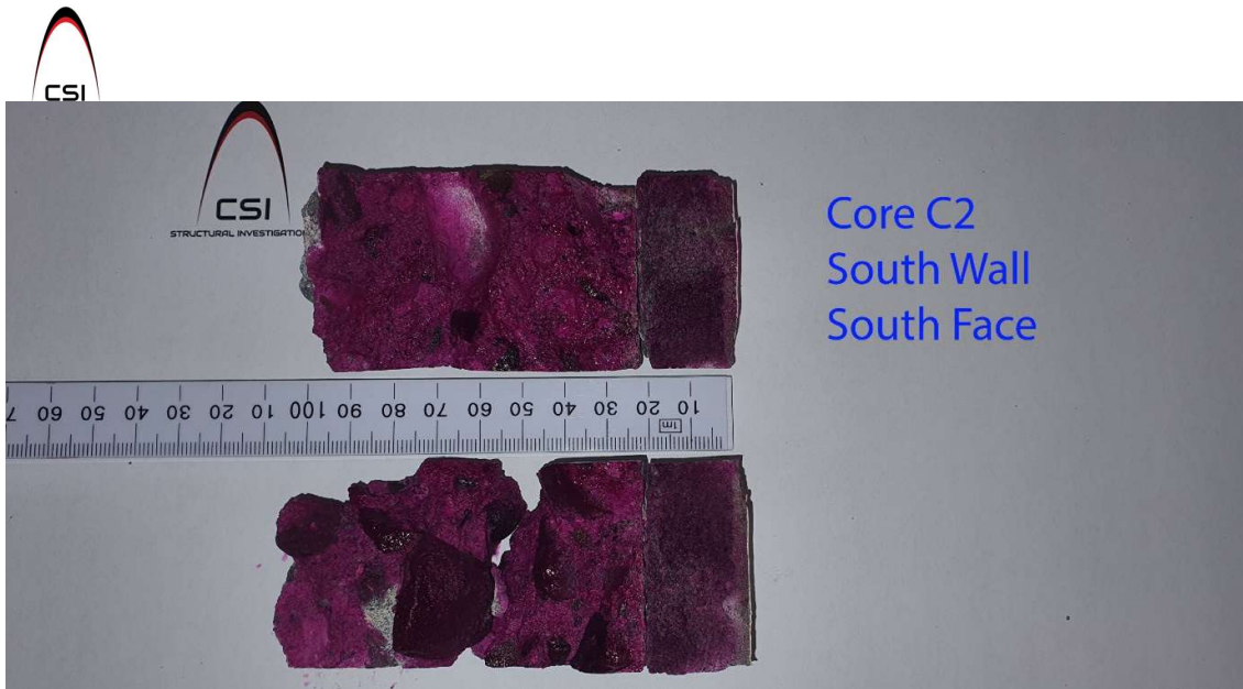
Figure 5: South Wall / South Face - Carbonation Testing
