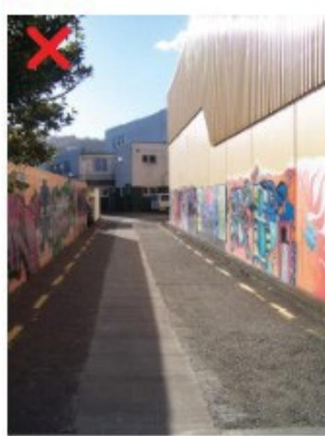
Unattractive side lane. The lack of public lighting, poor landscaping, blank walls and inactive uses on the ground floor increase the perception of insecurity
