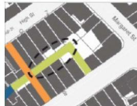
Movement corridor envelope is 3.5m wide x 4.5m high for one-way lane or 6.0m wide x 4.5m high for two-way lane (as a guide) - Eaves, balconies, planting or awnings should be carefully designed so as not to obstruct vehicle movement
