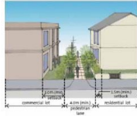
Transition 1 - Pedestrian Lane Side Boundary Interface
