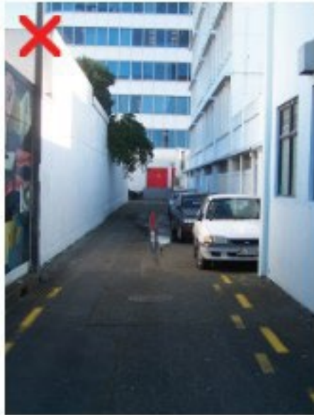
Rearlane is too narrow to allow for parking on one side. It obstructs trucks movement
