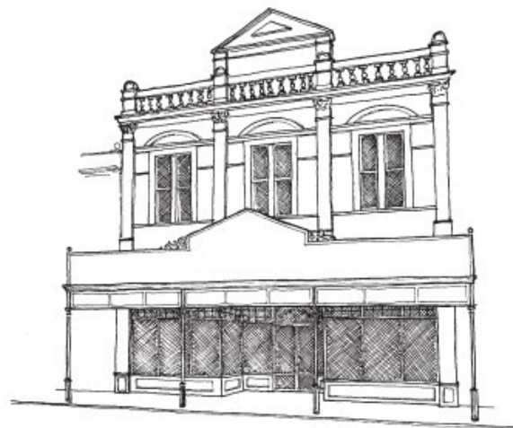
Building appears solid, windows built up to create depth. Shop front design reflects structural bays.
