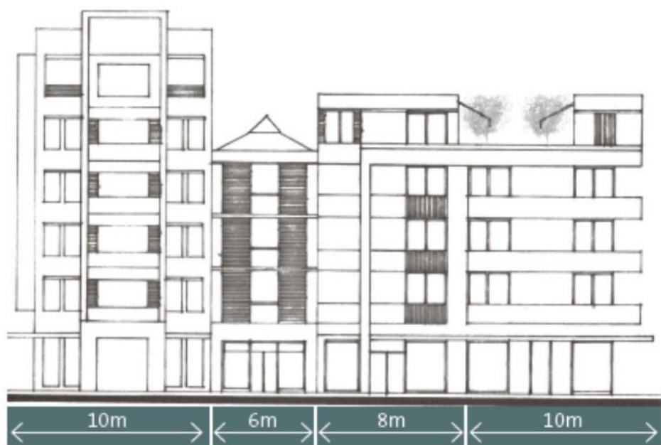
Example of a façade treatment in the Core Precinct. Long frontage lengths at intervals of less than 10m. Façade treatment of buildings (architectural elements and materials) on ground and upper floors at intervals of 2m to 6m to create interest to the streetscape.
