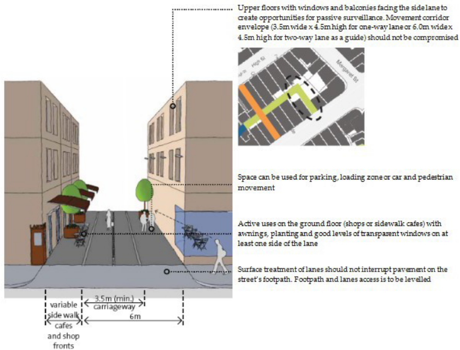
Side lane concept for the Central Area (the side of a building) Low-speed spaces with shared uses between pedestrians, cyclists and vehicles
