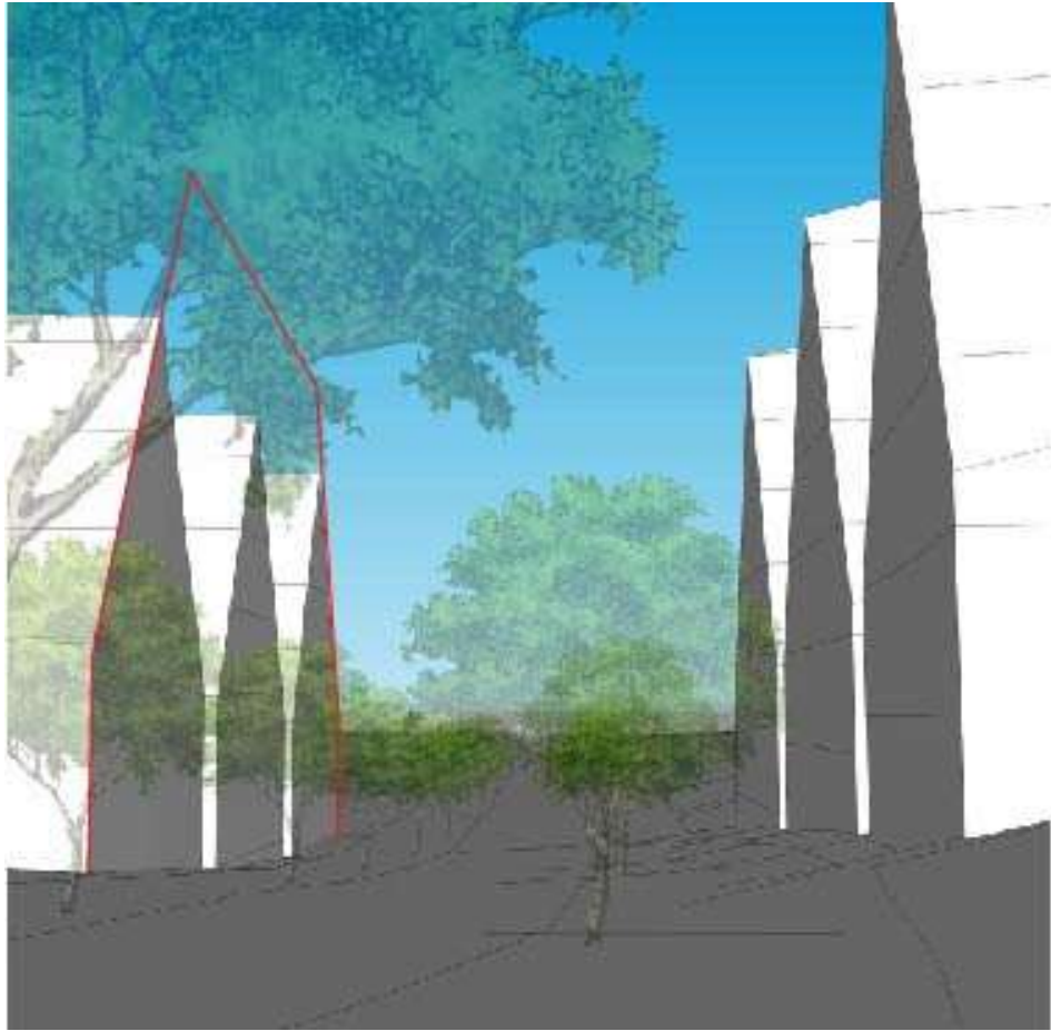
Figure 1 - An example of the bulk envelope (red line) of a site that is the result of amalgamating three sites, based on Attachment B, SK03 where the maximum height is not controlled by the HIRB and no internal HIRB control is applied.
