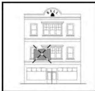
3. Sign conflicts with architectural features
