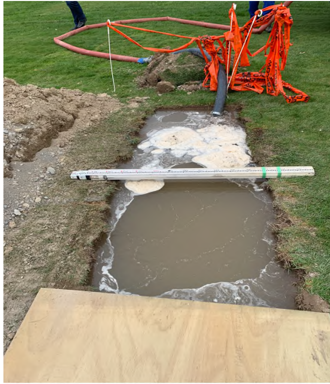
Above: View of soakage testing at test location 2
