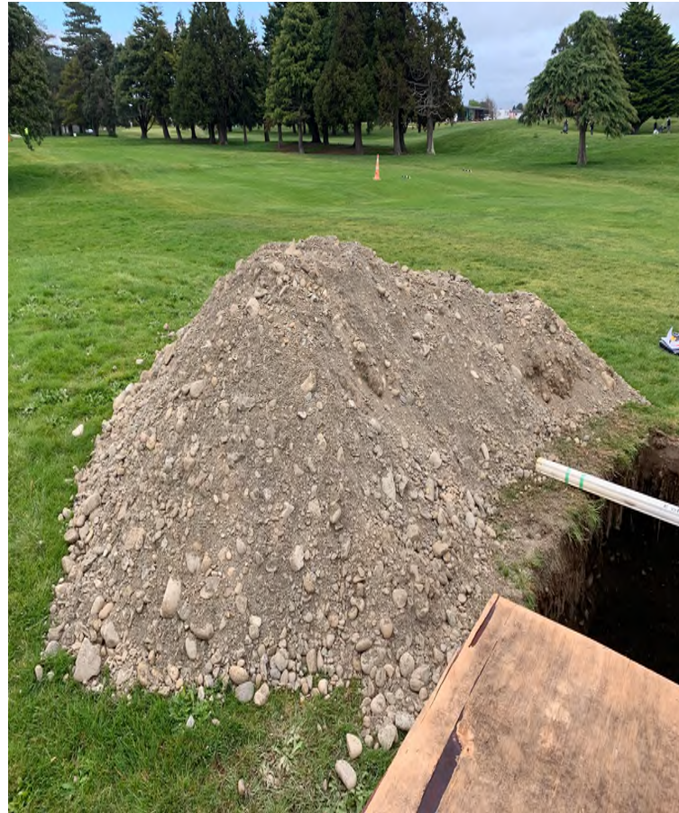
Above: View of excavated pit at test location 3 with material removed from ground shown
