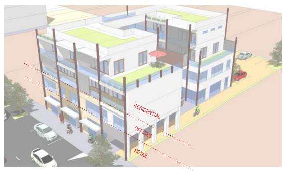
FIGURE 5.3.1 12m HIGH MIXED USE DEVELOPMENT INCORPORATING LOW IMPACT DESIGN SOLUTIONS
