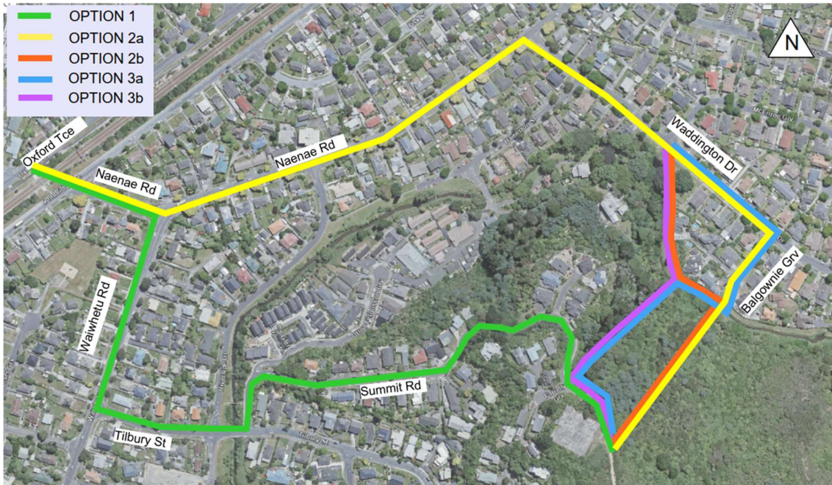
Figure 2: Delivery pipe alignment options (Options 2b, 3a and 3b only shown up to where all join a common alignment with Option 2a on Waddington Drive)
