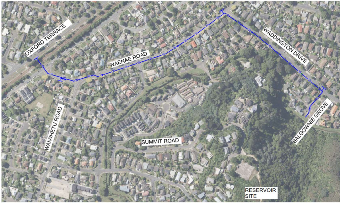
Figure 2: Delivery pipe alignment
