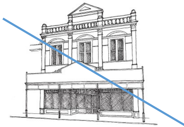
Building appears solid, windows built up to create depth. Shop front design reflects structural bays.
