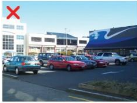
Poor landscaping - lack of trees, shrubs and permeable paving
