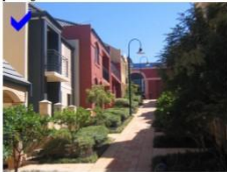
Pedestrian lane in medium-density residential developments. Good public lighting, balconies and windows facing the footpath, low and transparent fencing, high quality paving and planting and pedestrian entry to the dwellings
