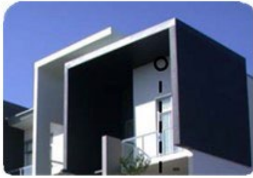
Horizontal shading device (overhangs) on north facing
