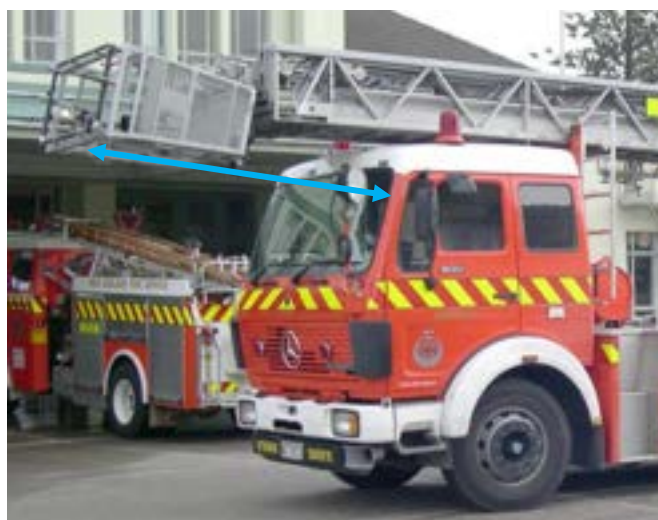
Figure 5 – Showing long front overhang
