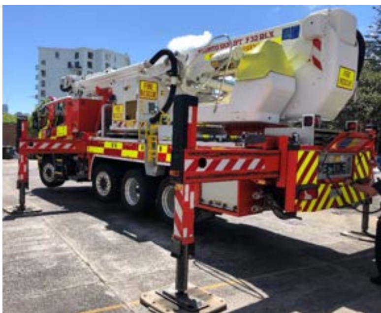
Figure 13 – Highlights the space requirements for jacking stabilisers
