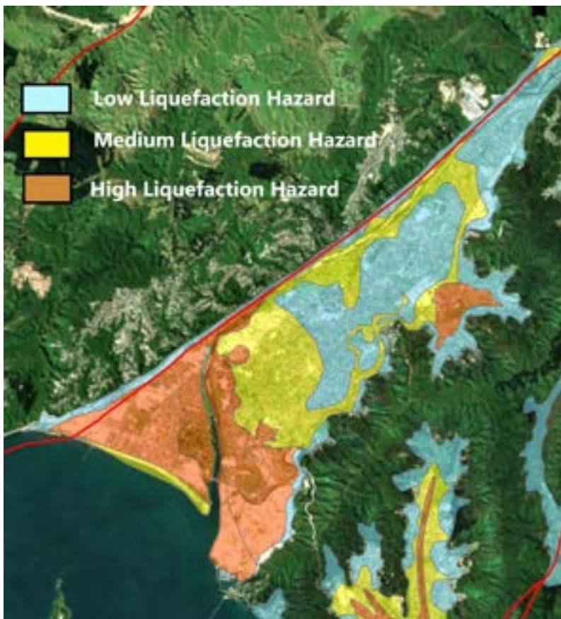
Figure 1: Liquefaction susceptibility map showing high (orange), medium (yellow) and low (blue) susceptibility to liquefaction in Lower Hutt. Data from Greater Wellington Regional Council
