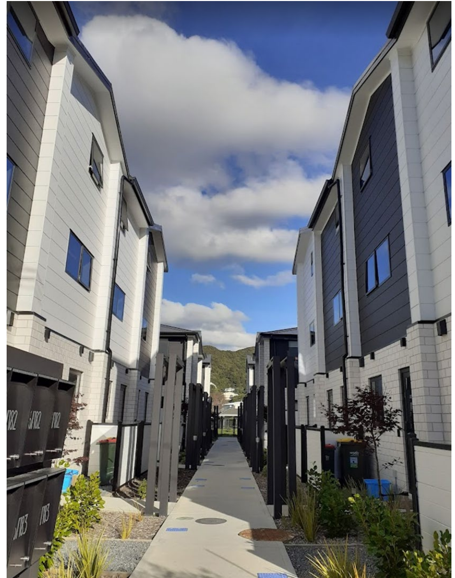
A Hutt City example in Cambridge Tce: Hard surfaces, minimum permeable surface, minimal spaces for larger shade trees, maximum reflectivity. In winter, the opposite effect due to shading (tight proximity / canyoning) is possible (also wind tunnel effects).
