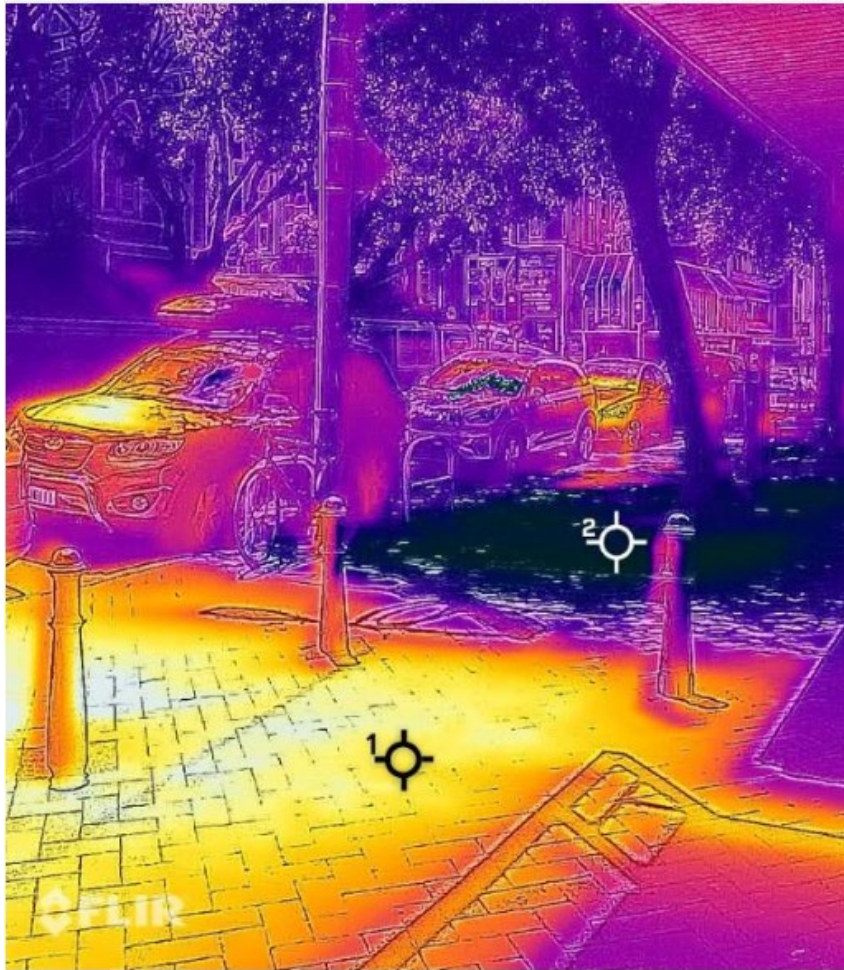
This image, captured with an infrared camera, reveals the surface (not air) temperature on a sunny summer afternoon in January on a treelined street in central Wellington. The yellow areas are hotter surfaces, and the blue/black areas are cooler. The air temperature was 23 °C. The surface temperatures at two locations are shown at the top left of the image. The pavement in full sun is 47.7 °C whereas the ground under the tree is 20.3 °C.
