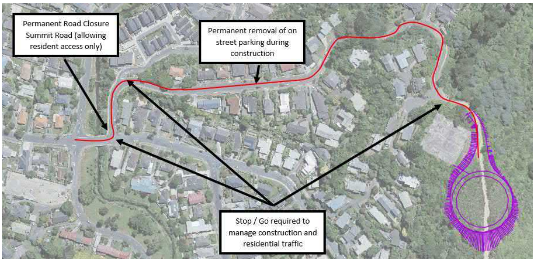
Figure 6 - Traffic Management for Naenae Reservoir
