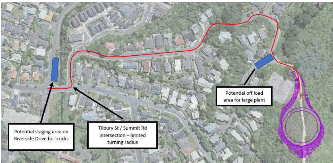
Figure 4 - Access route to Naenae reservoir site
