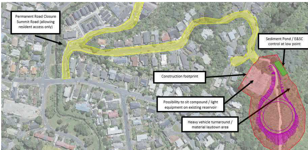
Figure 5 - Site footprint of Naenae reservoir site
