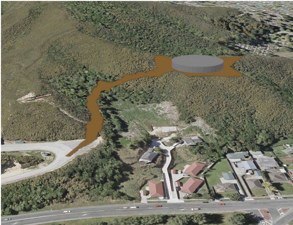
Figure 35. Indicative view of Cambridge Terrace site (brown shading indicates extent of earthworks)
