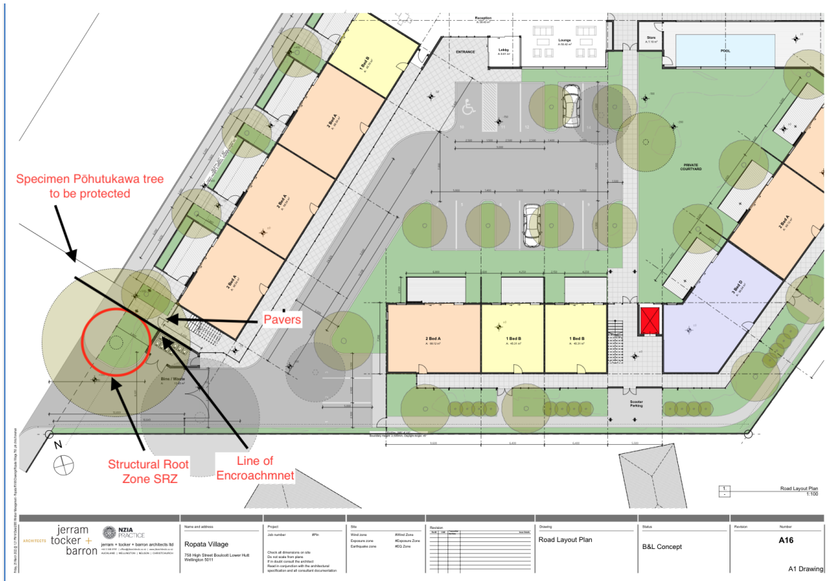
Appendix 19: The line of encroachment for the paved area breaches the TPZ but not the SRZ, so long as the non-woody roots are kept moist and cool and the finish height of the pavers is no different to the original heights, minimal recommendations are suggested
