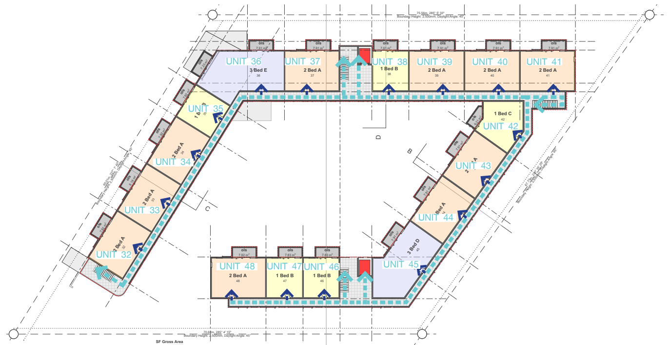
Figure 23: Circulation diagram - second floor (Pedestrian primary - light blue, pedestrian secondary - dark blue)
