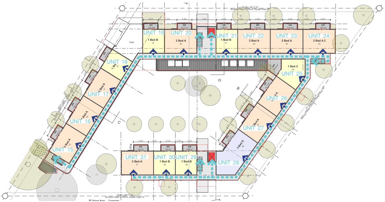
Figure 22: Circulation diagram - first floor (Pedestrian primary - light blue, pedestrian secondary - dark blue)
