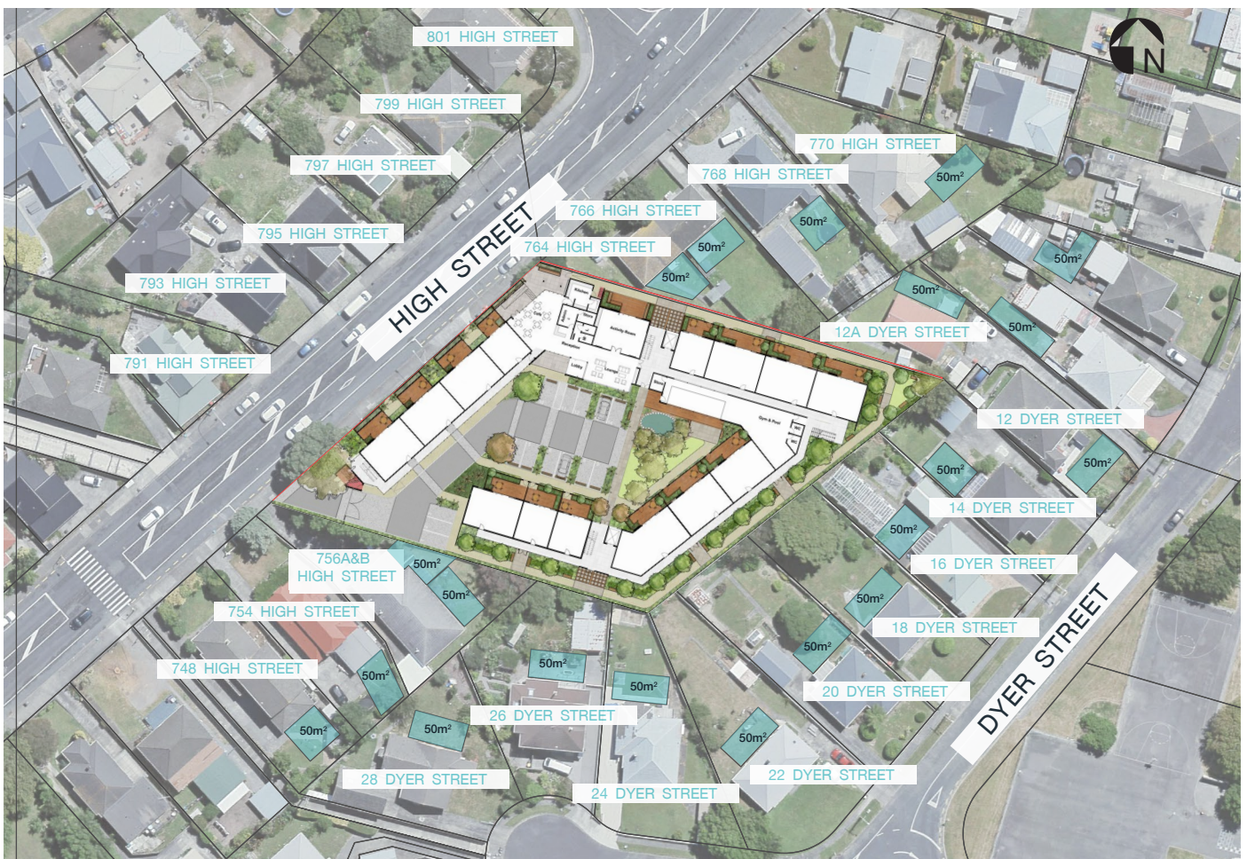
Figure 6: Neighbouring Properties Map - 50m² outdoor areas of neighbouring properties shown in blue
