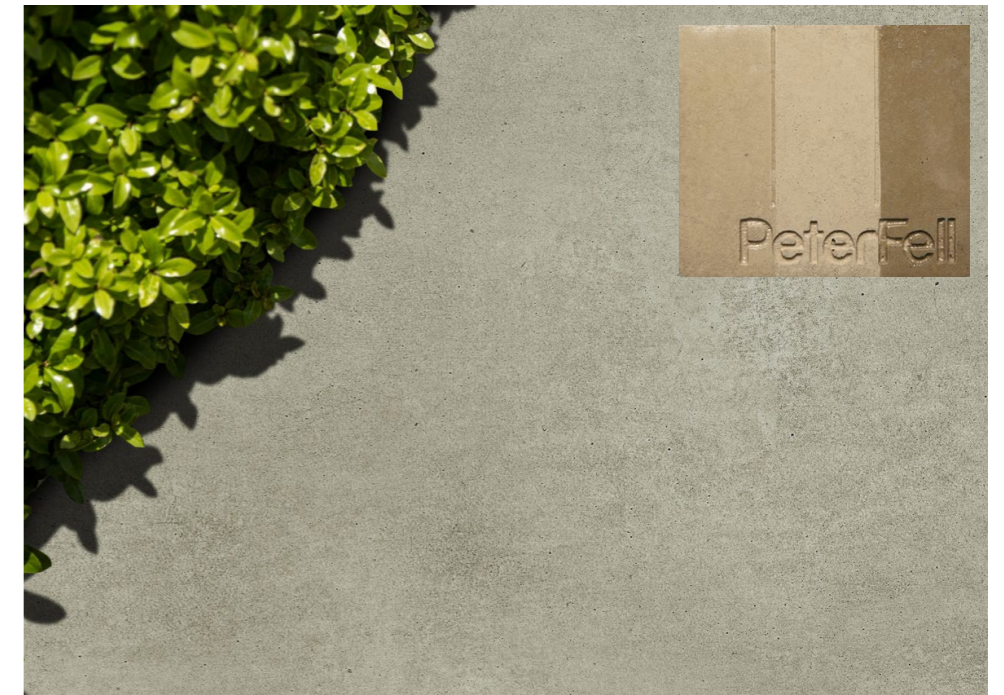
(C) Coloured Concrete - 'Peter Fell colour oxide 167®' or Firth 'Sea breeze®' or similar approved - decorative saw cuts to be included and specified in detailed design
