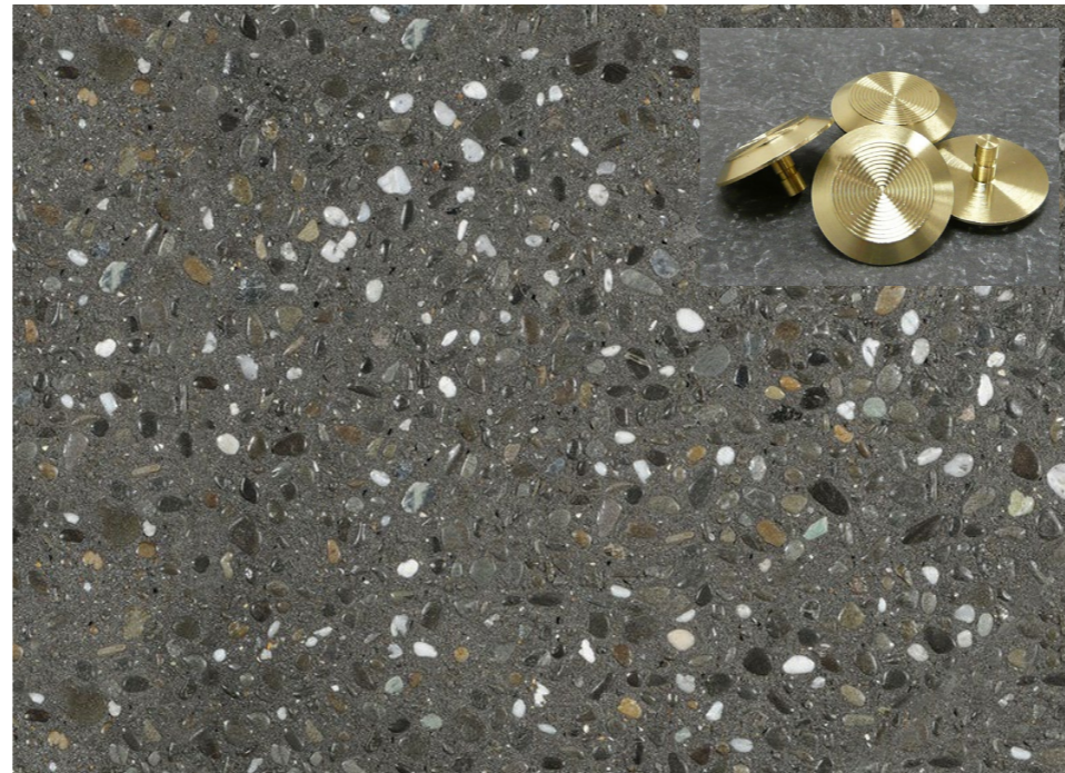
(B) Exposed aggregate concrete - 13mm Rangitikei River pebble aggregate with 5% black oxide or similar contrasting material. Brass tactile stud delineation between carparks - 200mm spacing
