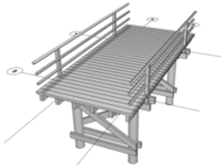
Figure 35. A representative bay of the approach portion of the wharf as built in 1908. Original fabric is grey.
