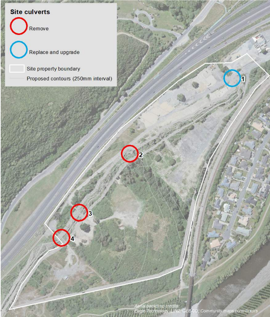
Figure 2 Culvert option, October 2022: removal and replacement
