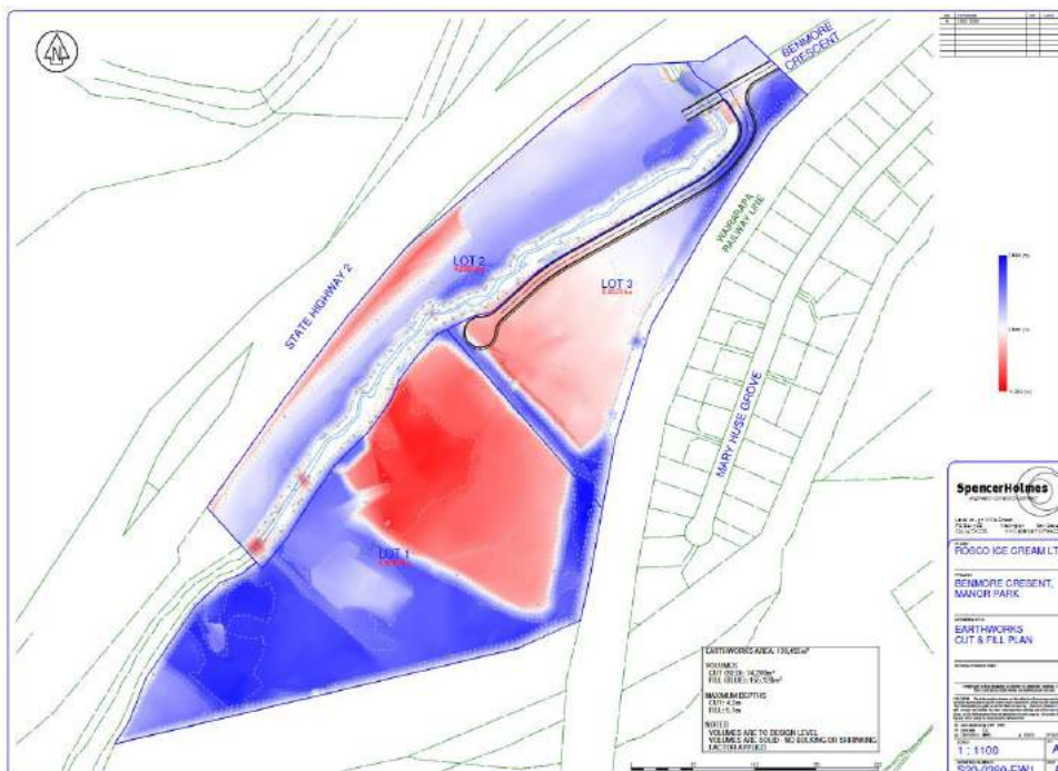
Figure 1. Earthworks Cut and Fill Plan
