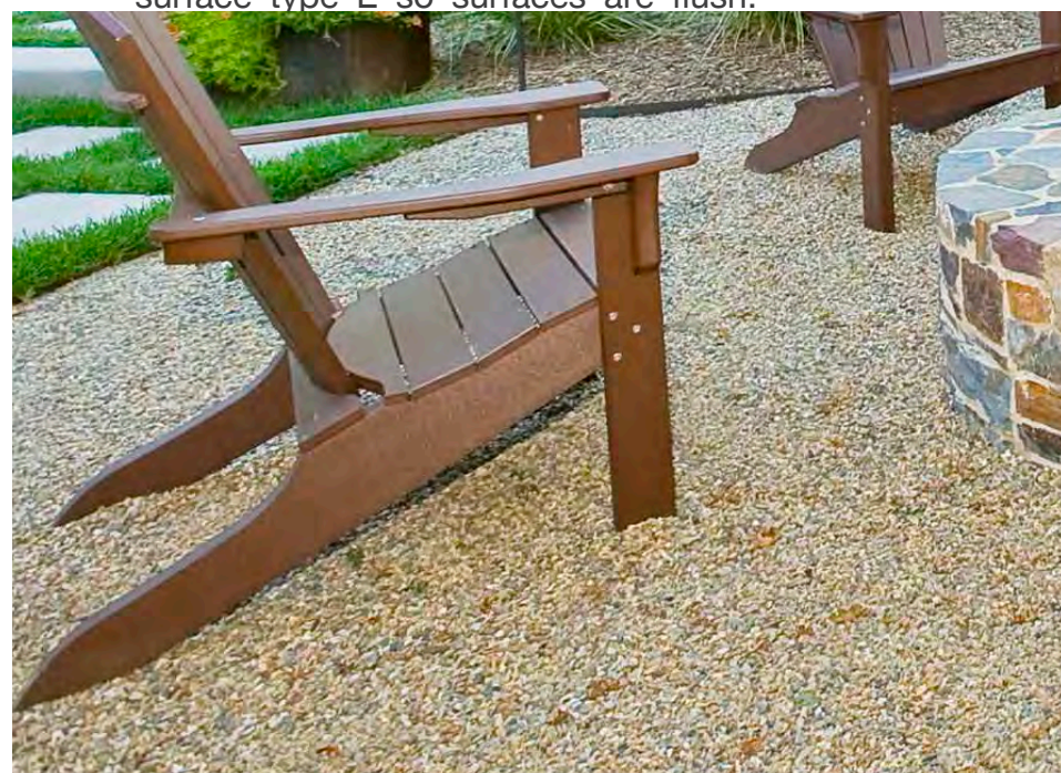
Ⓔ Surface E - Reinforced gravel or compacted lime chip. 20mm river pebbles over subsurface stabilisation mat or compacted lime chip.
