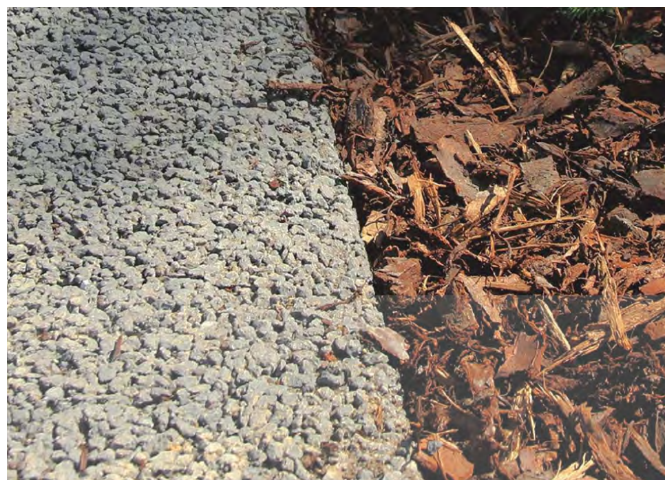
Ⓐ Surface A - Permeable concrete. Firth perm-con. Saw cuts to be specified at detailed design stage. (Or similar approved permeable concrete surface).
