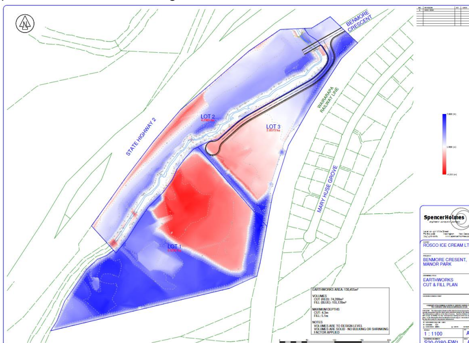
Figure 1. Earthworks Cut and Fill Plan
