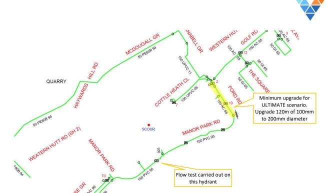
Figure 10 - Potential mains requiring upgrade for ULTIMATE solution.
