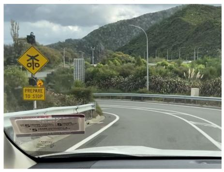
Figure 3-8: Curved Approach Limiting Forward Visibility of Crossing
