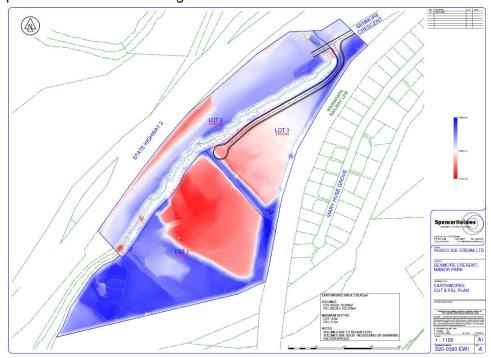
Figure 1. Earthworks Cut and Fill Plan
