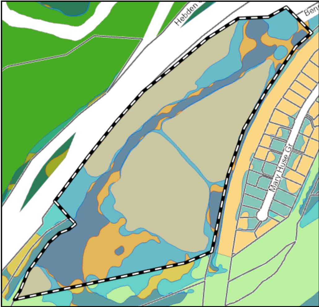
Figure 13: Application site with High (dark blue), Medium (orange) and Low (light blue) Flood Hazard Overlays under the PDP
