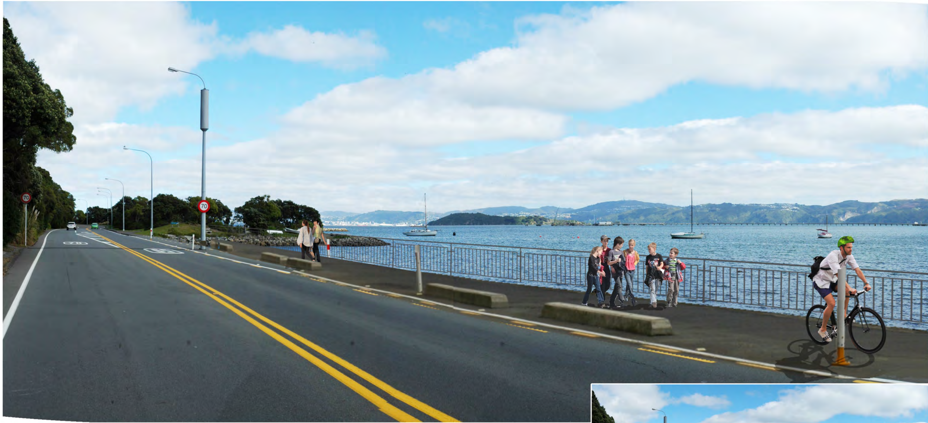
Simulated view of proposed 3.5m wide shared path with safety railing on the southern section of Lowry Bay looking south west, along Marine Drive towards Whiorau Reserve
