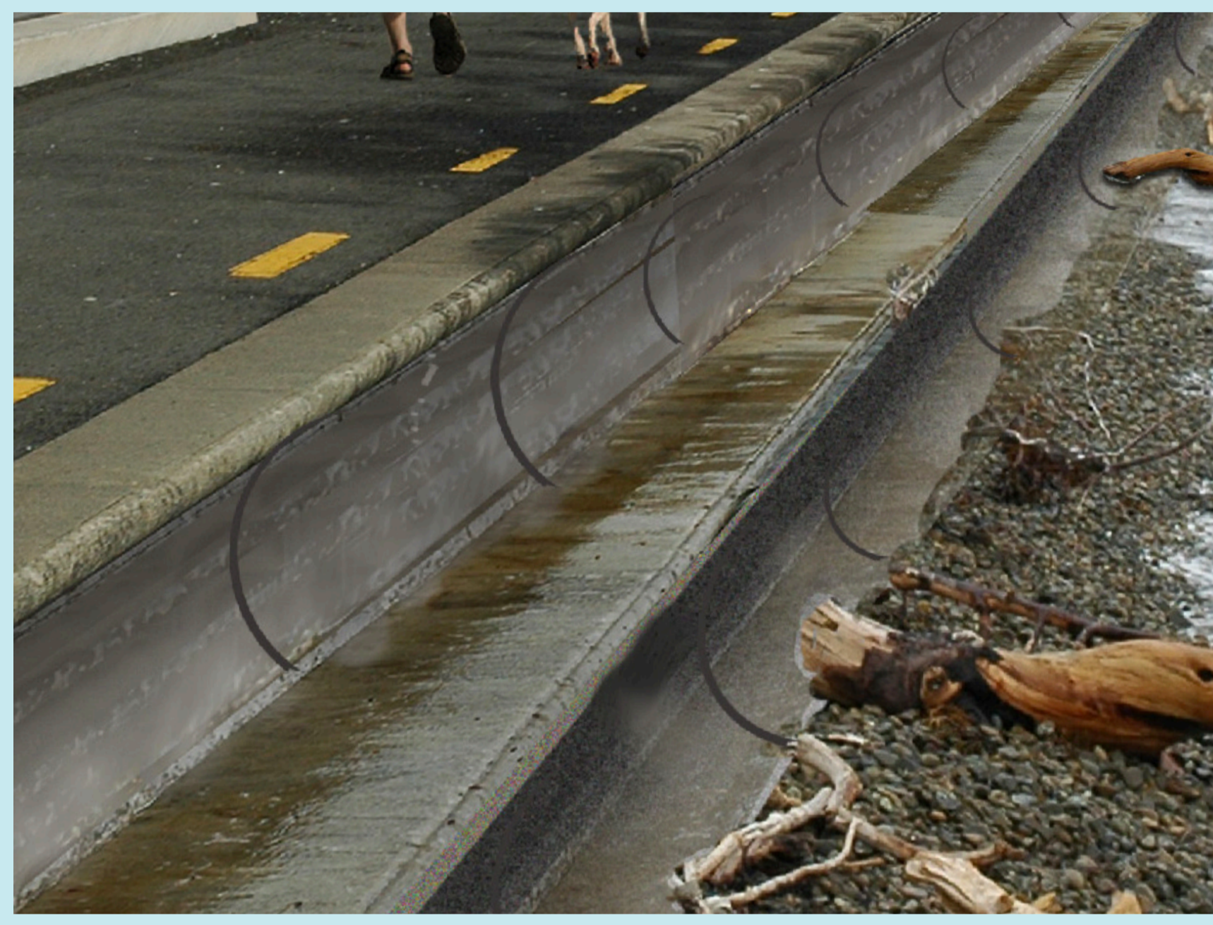
Indicative shape of curved seawall design
