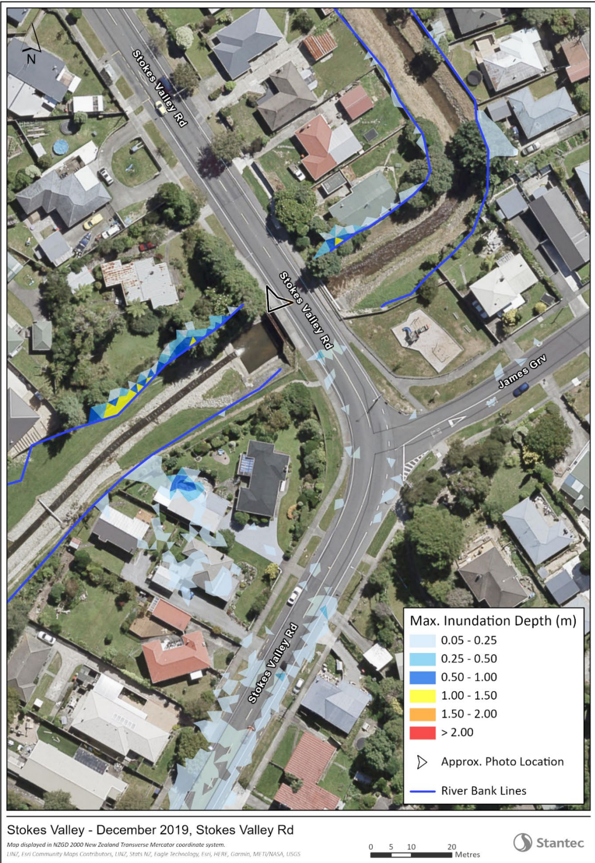
Figure 4-4: Modelled Flooding of the Stokes Valley Stream at Stokes Valley Road.
