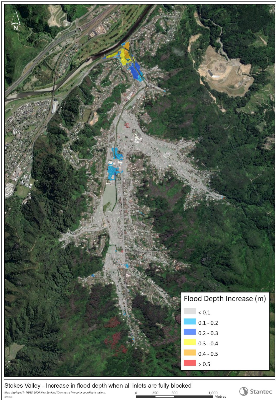
Figure 5-2: Difference in depth between the 100yr ARI with climate change scenario and the 100% blocked scenario.
