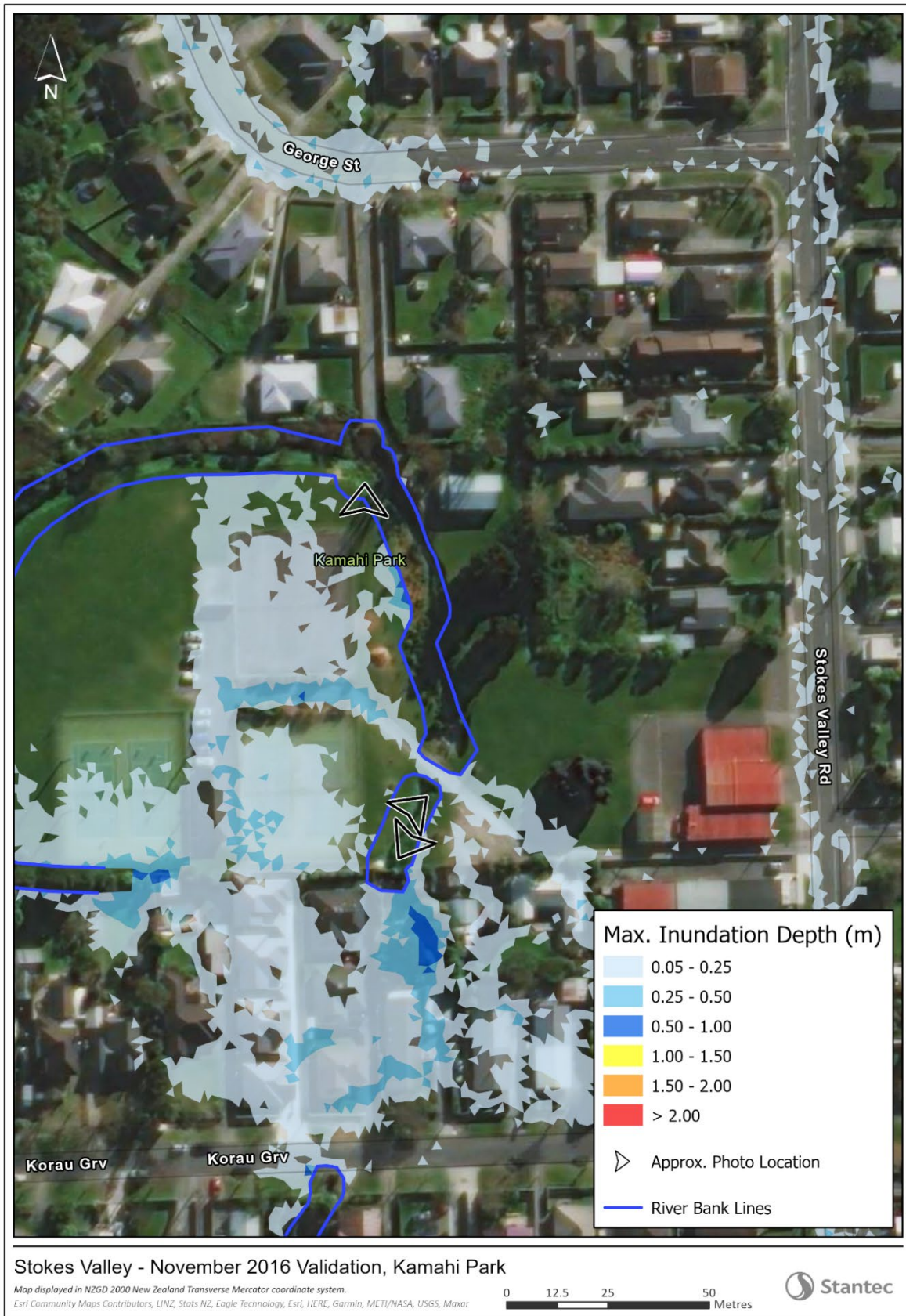
Figure 4-47: Boundary of the modelled 1D channel (blue line) and maximum 2D flood depths near Kamahi Park (15 November 2016 event)
