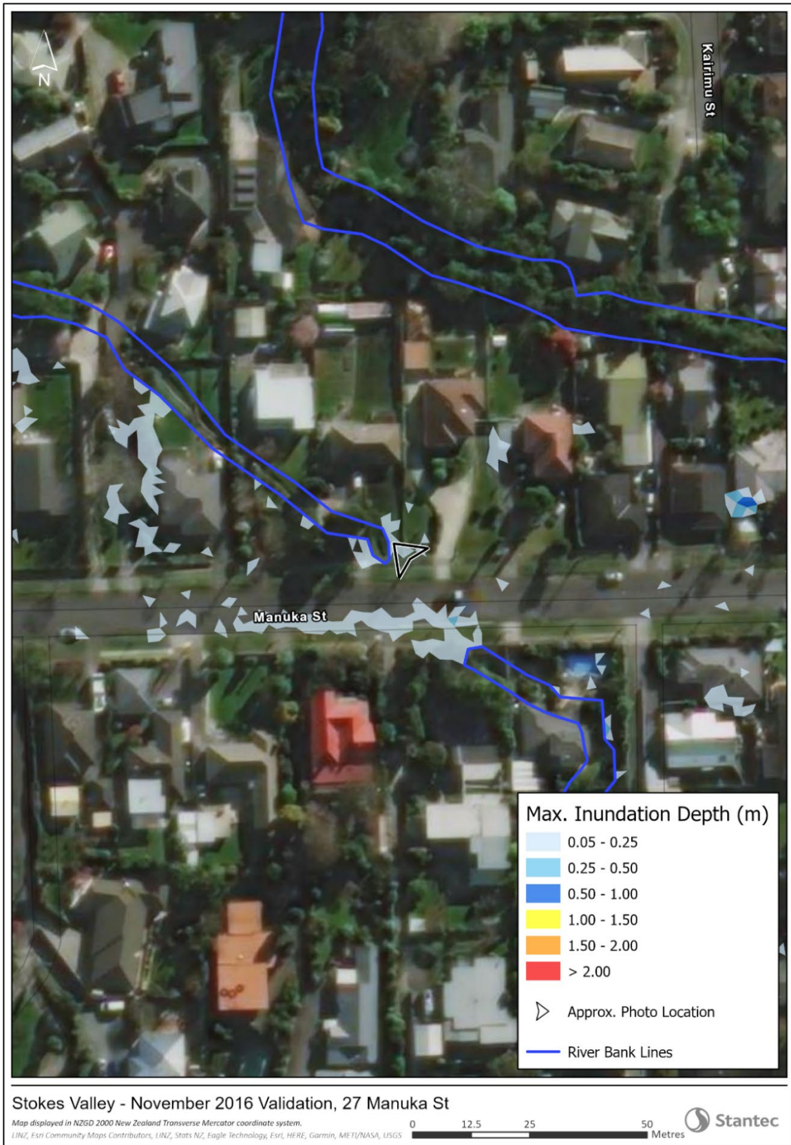
Figure 4-54: Boundary of the modelled 1D channel (blue line) and maximum 2D flood depths at 27 Manuka Street (15 November 2016 event).
