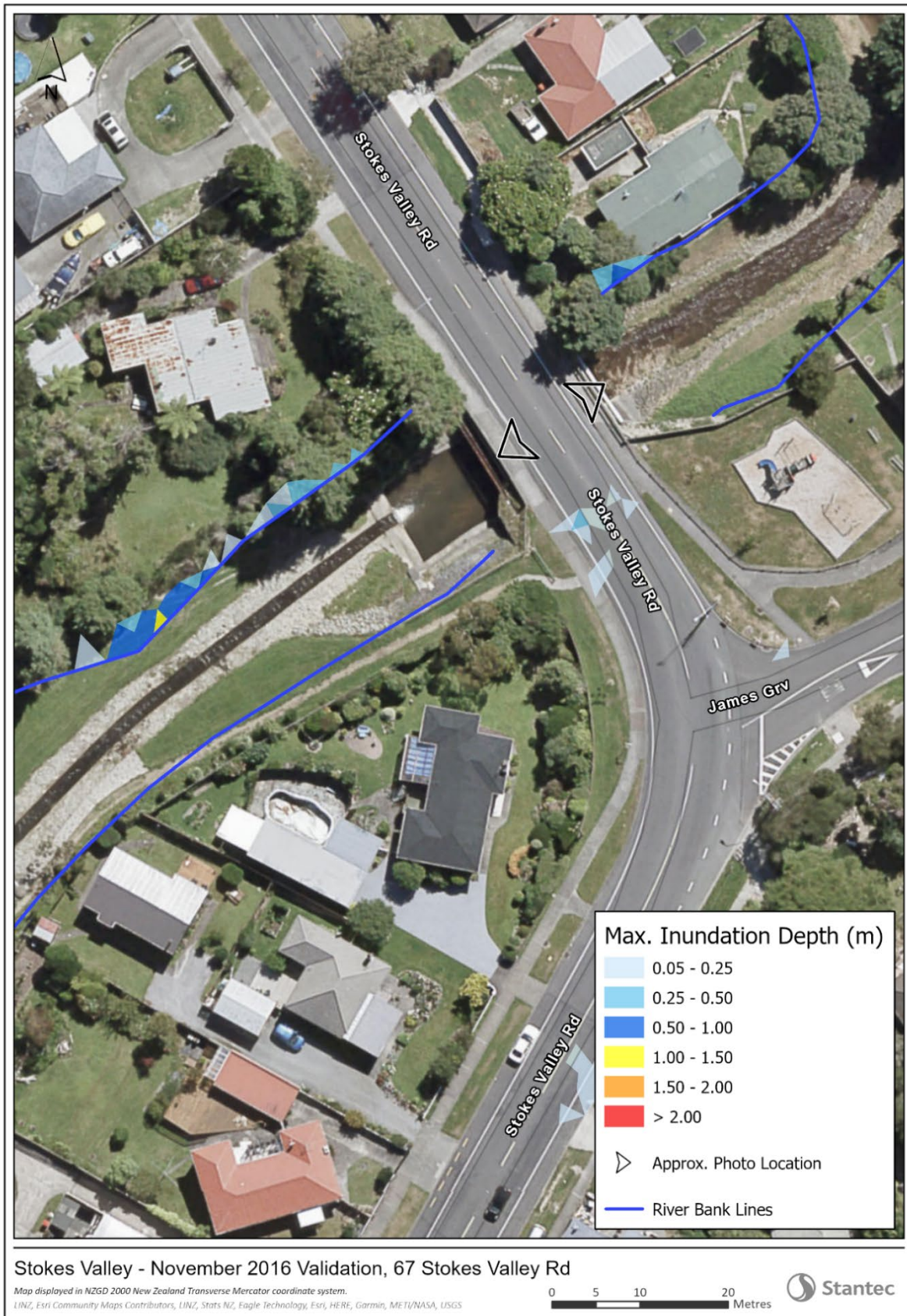
Figure 4-27: Boundary of the modelled 1D channel (blue line) and maximum 2D depths near 67 Stokes Valley Road (15 November 2016 event).
