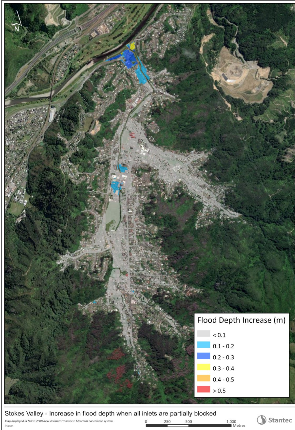
Figure 5-3: Difference in depth between the 100yr ARI with climate change scenario and the 50% blocked scenario.
