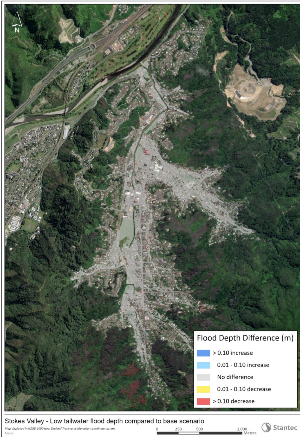
Figure 5-4: Difference in depth between the 100yr ARI with climate change scenario and the low tailwater scenario.
