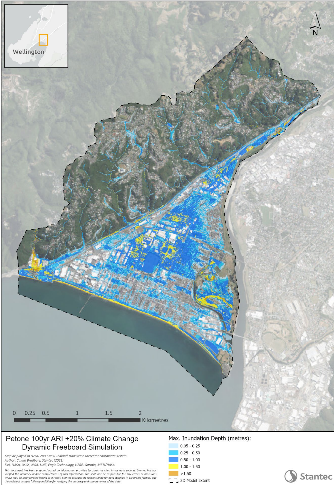
Figure 6-9 Maximum flood depths for the 100y ARI + 20% CC design event including dynamic freeboard
