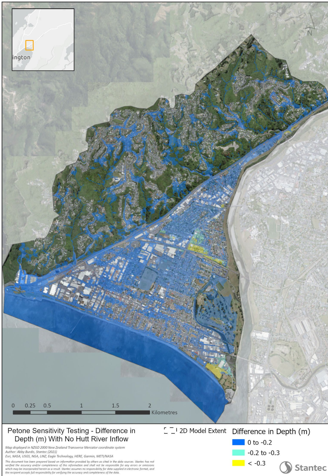
Figure 6-6 Difference in depth between the base case scenario and a simulation with the Hutt River inflow removed
