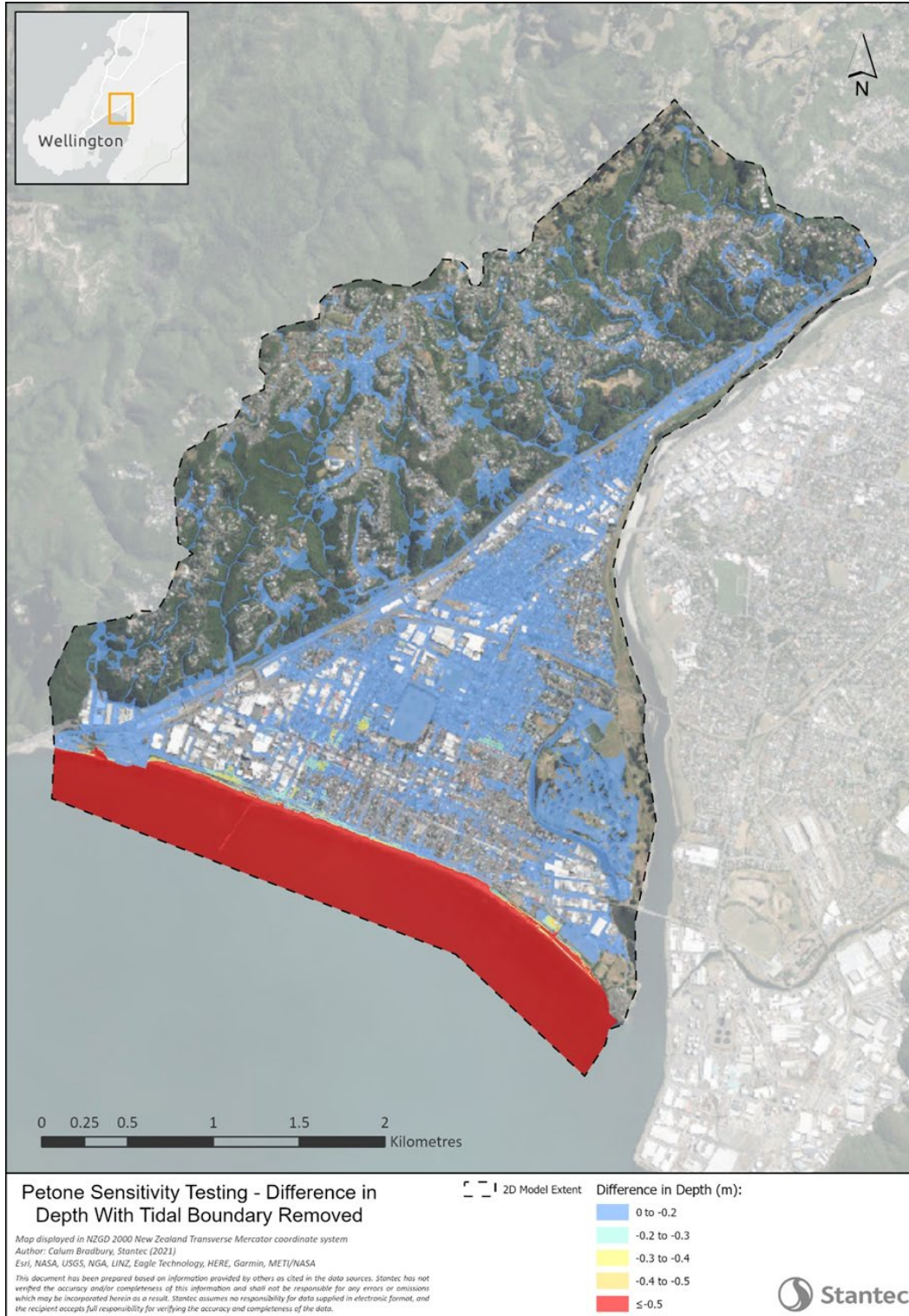
Figure 6-5 Difference in depth between the base case scenario and a simulation with the tidal boundary condition removed
