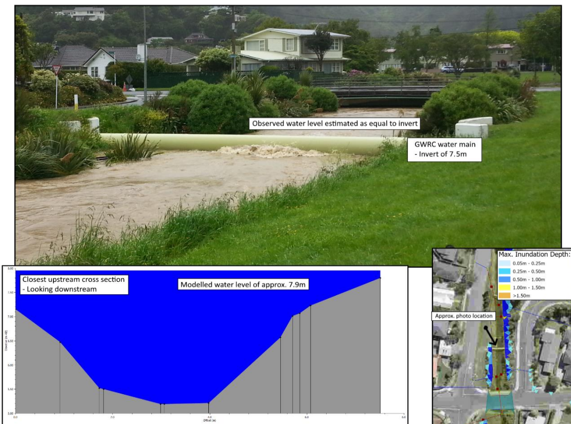
Figure 6-27 Observed and modelled stream levels at the Tilbury Street bridge (downstream).
