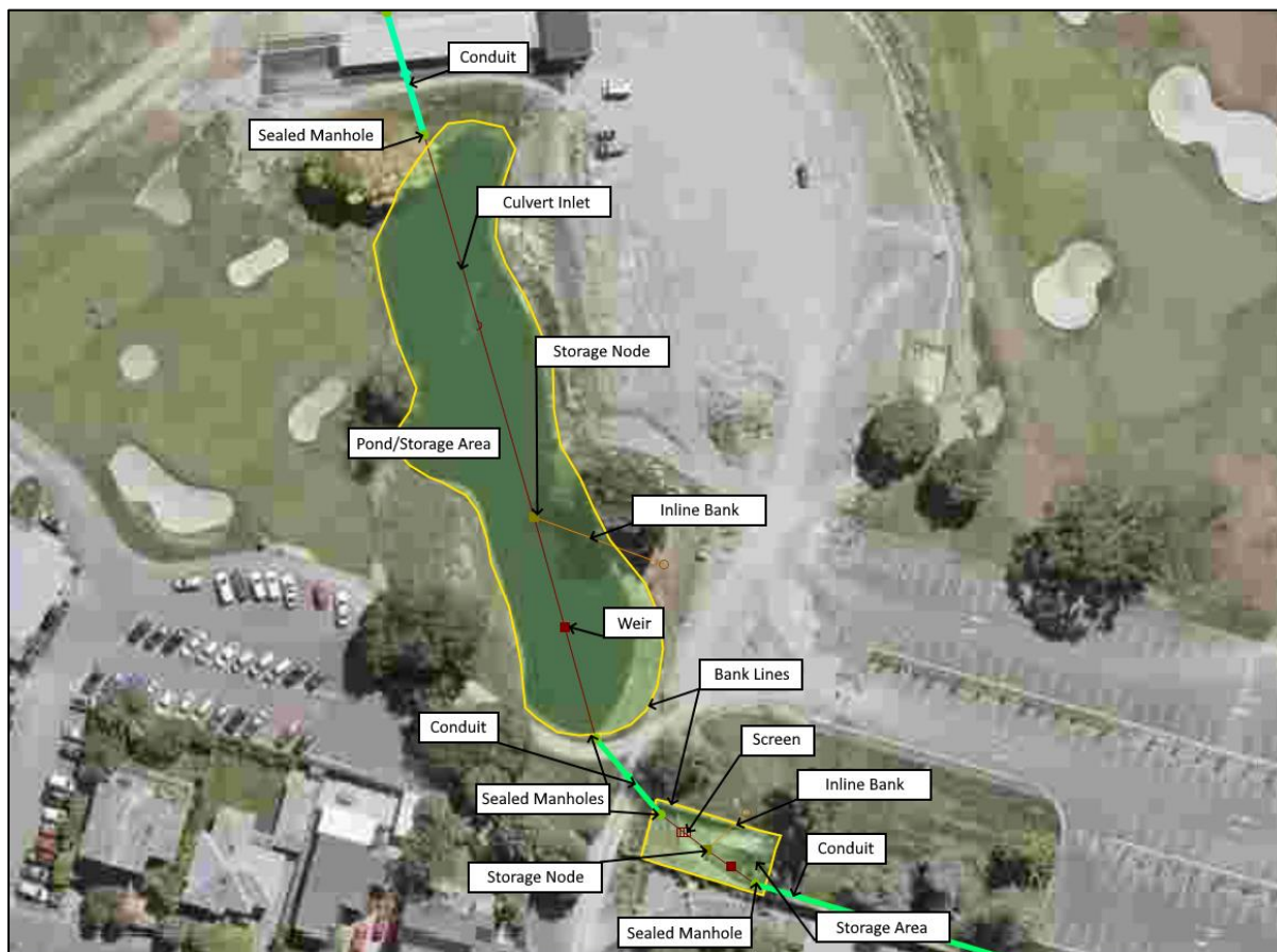
Figure 3-7 Overview of 1-D pond construction.
