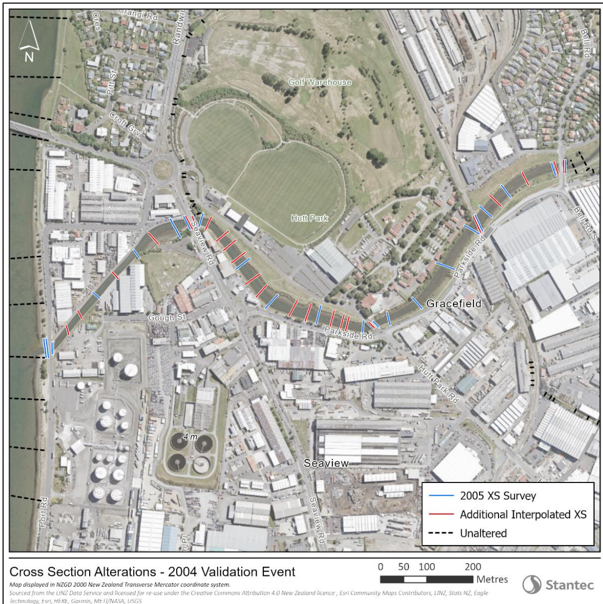
Figure 5-2 Cross sections altered to account for the 2009-2010 Waiwhetū channel improvements.
