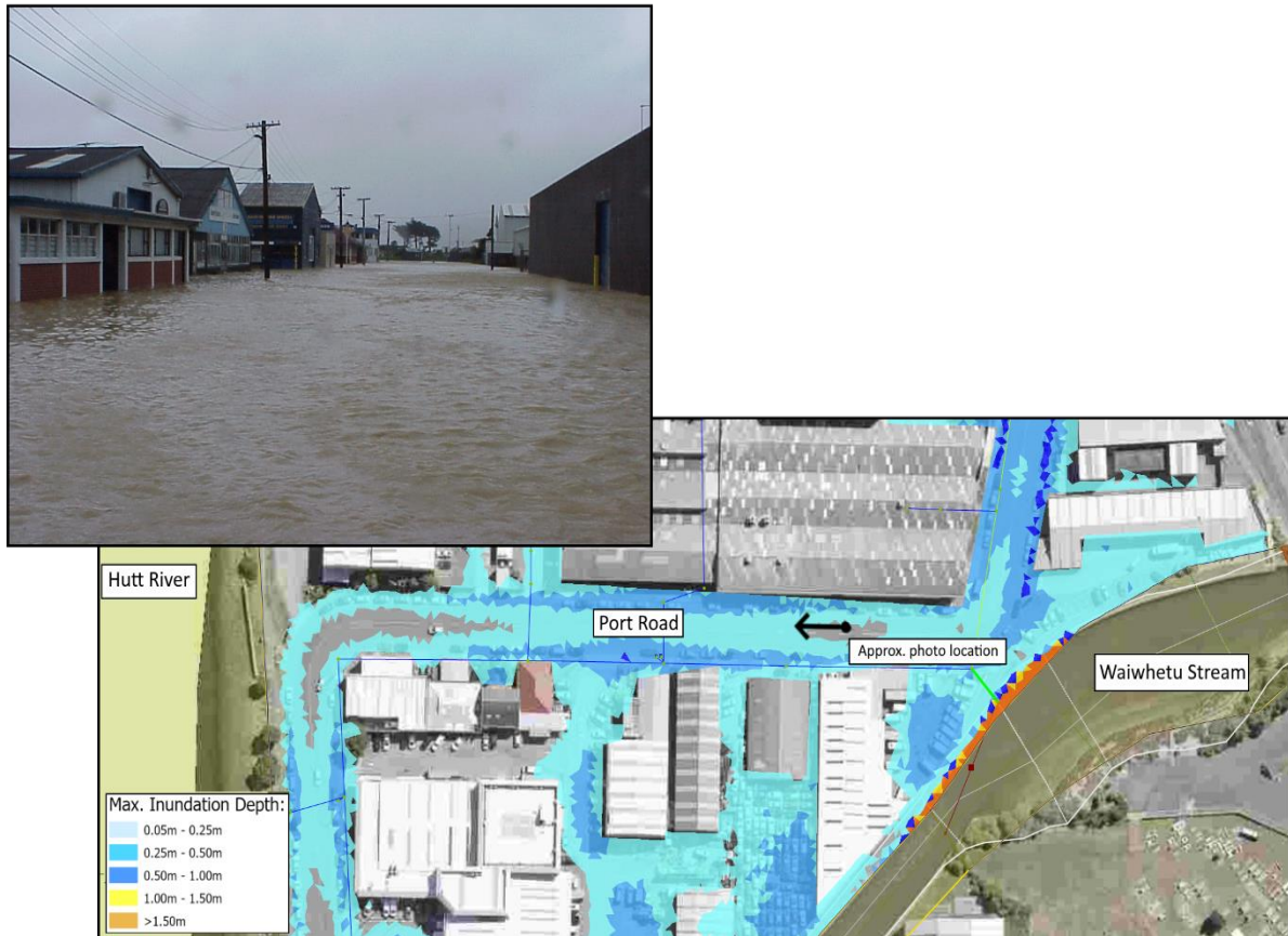
Figure 6-9 Photo of flooding facing west at 6 Port Road combined with model simulation extents.
