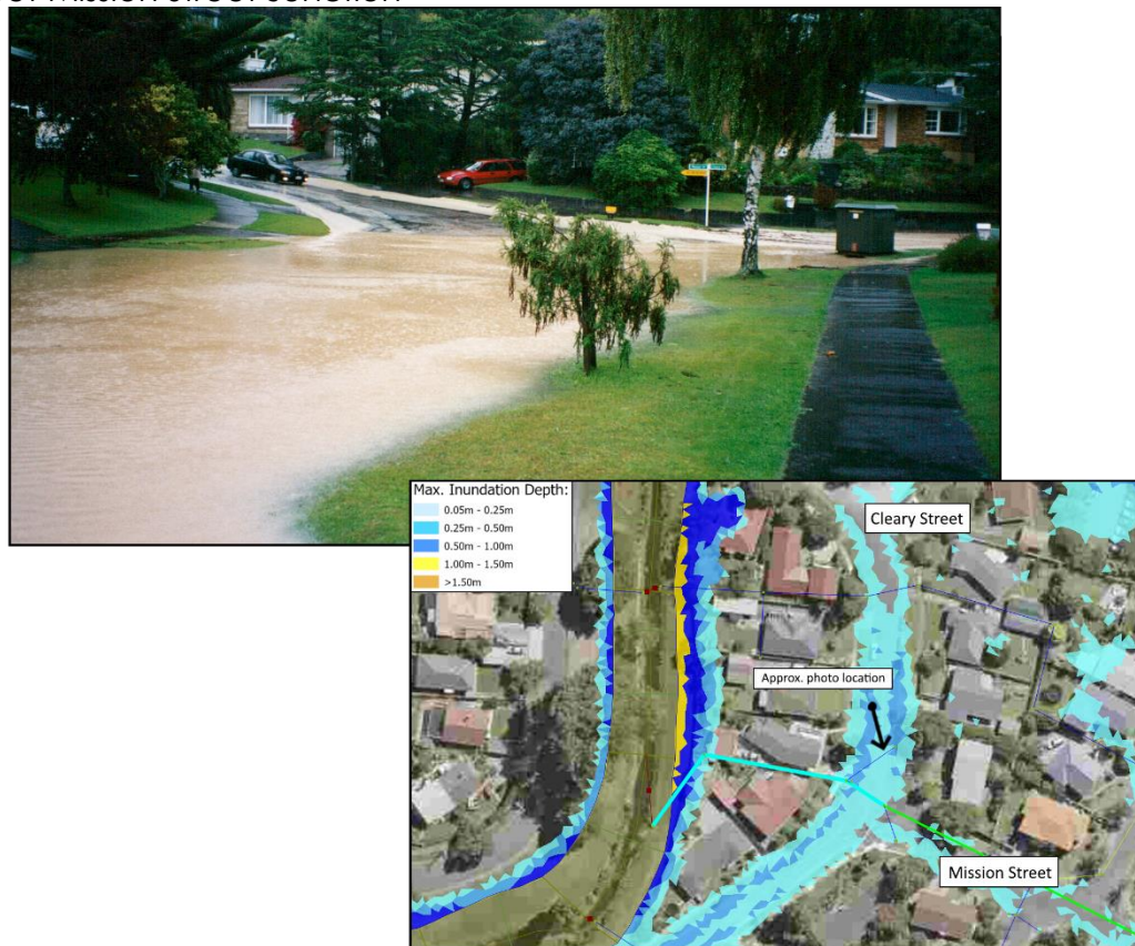
Figure 6-12 Photo of observed and modelled flooding extents at the Cleary Street-Mission Street Junction.
