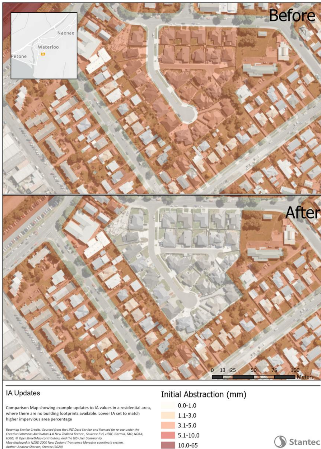
Figure 3-2 Initial abstraction is reduced to account for construction of new residential housing, and an associated increase in impervious area.
