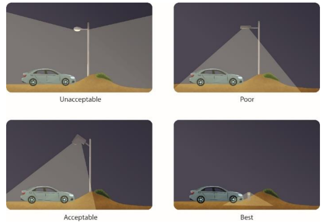
Figure 5 Lighting options for a parking area. Figure adapted from Witherington and Martin (2003) 3 .
