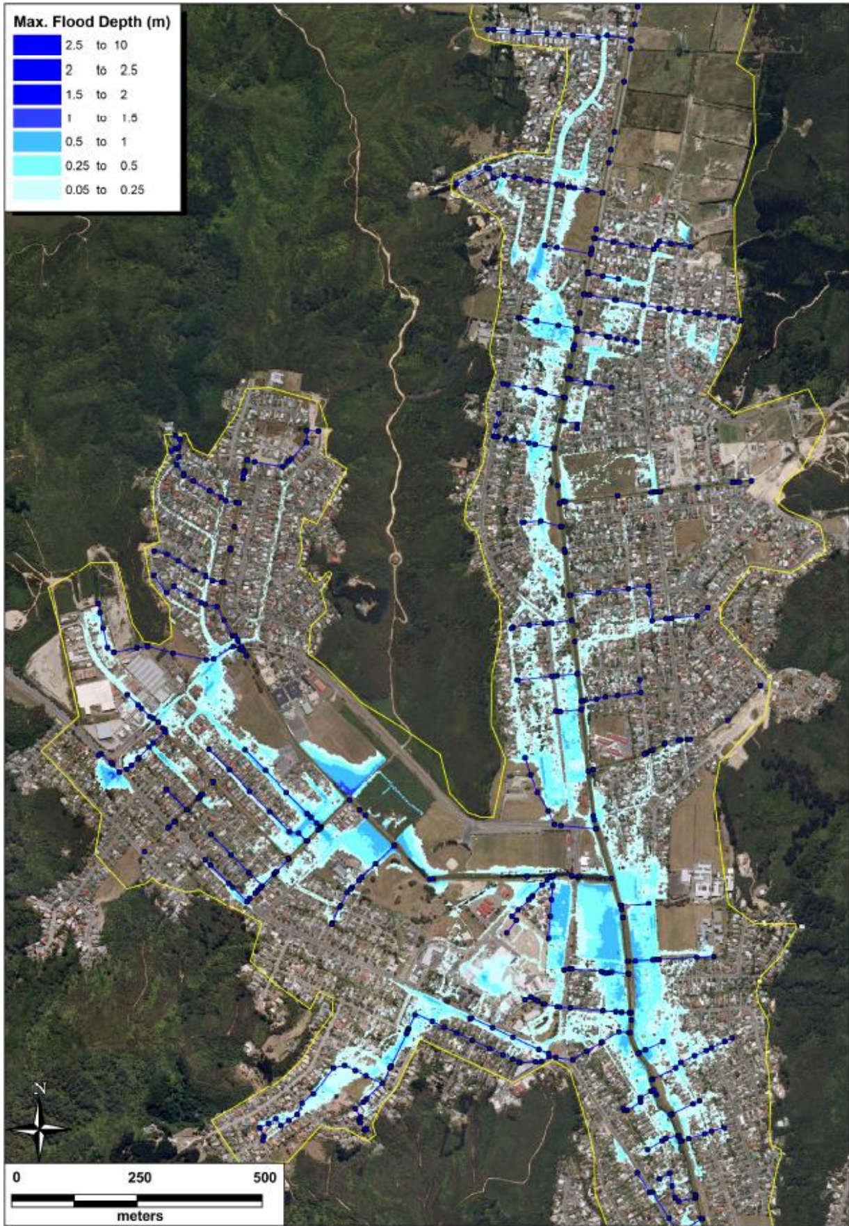
Figure 10-41: Maximum flood depths during the 50yr ARI event under future climate conditions – pre development
