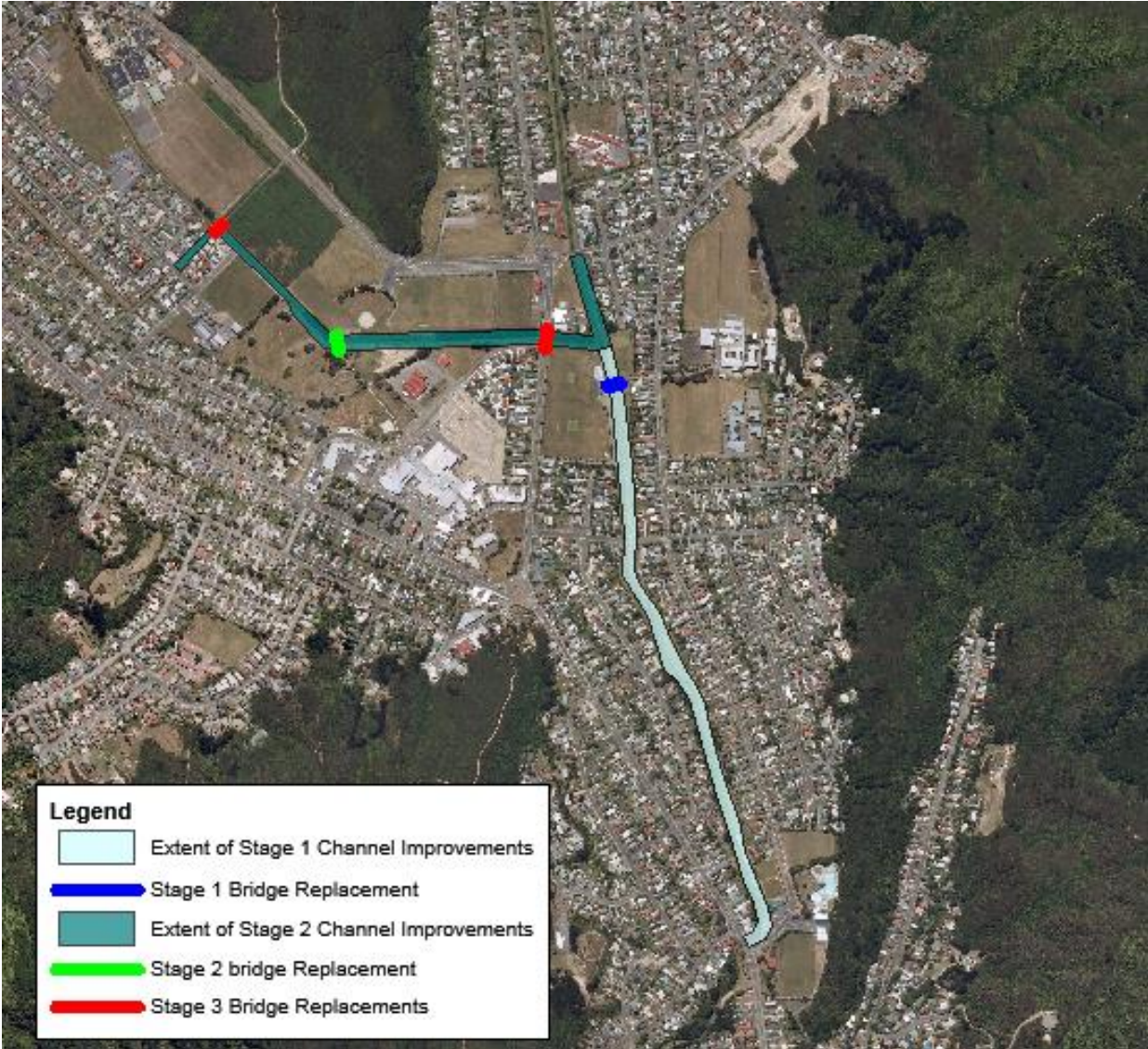
Figure 3-8: Extent of the channel improvement works carried out between 2004 and 2009
