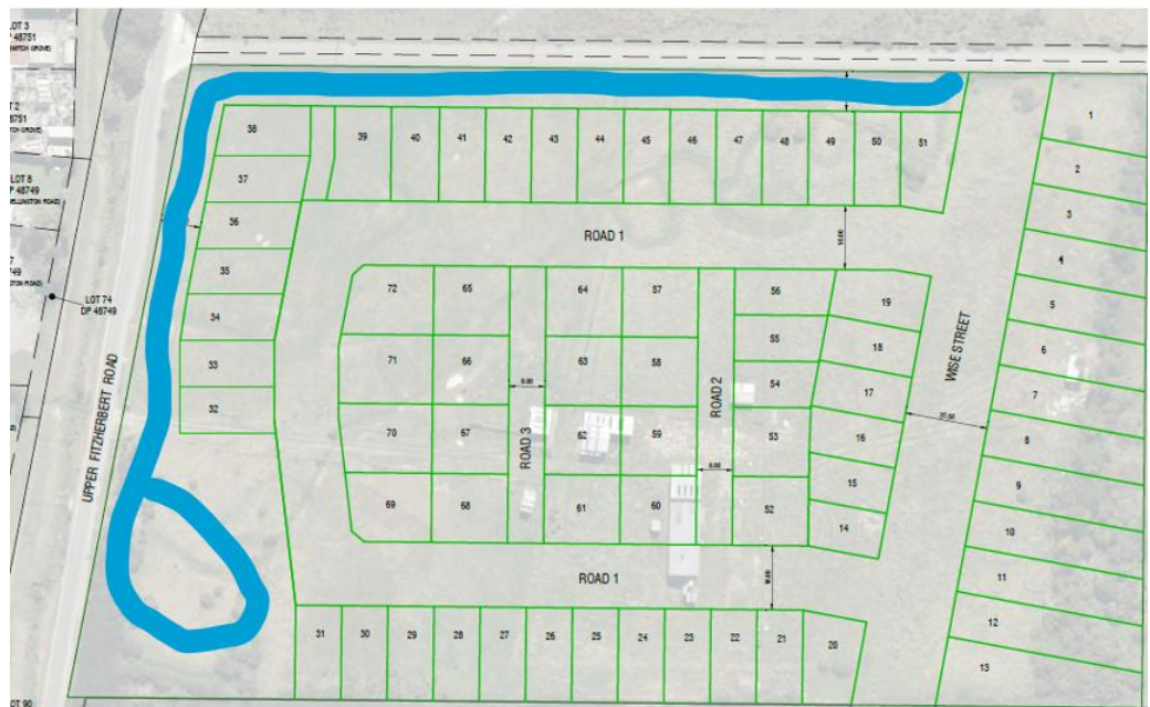
Figure 3 Possible development layout. My blue line indicating wetland swale and wetland retention basin opportunities.
