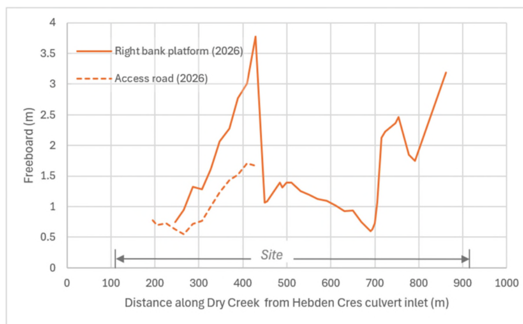
Figure 3: Predicted freeboard, 1% AEP flood (RCP 8.5 2130), current (2026) situation
