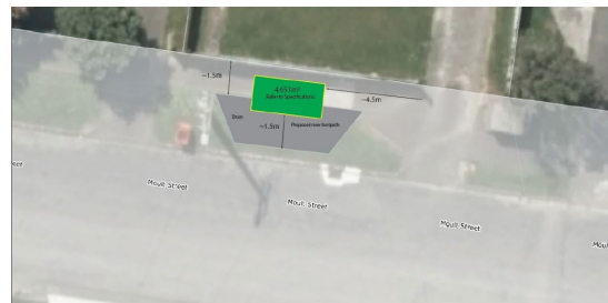
Figure 1: Existing transformer location and proposed replacement position at 9 Moul Street, Tītahi Bay. Source: WELL / Align resource consent material, April 2026.
