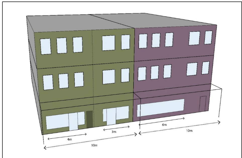
Figure 1: Left (compliant) has 70% glazing with only 40% continuous, to enable a finer-grained proposal with two store fronts and apartment access. Right (non-compliant) has 60% continuous glazing and there is no 3m featureless facade infringement due to door.
