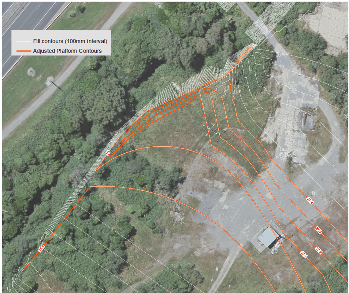
Figure 7 Amendment of fill platform
