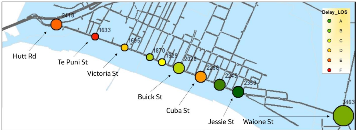
Figure 10 Intersection Performance (AM Peak)
